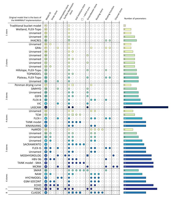
Figure 2: Overview of MARRMoT models. Models are sorted vertically by number of stores (1 at the top, 8 at the bottom). The columns show broad categories of hydrologic process that can be represented by a model. Coloured circles indicate the model has a store dedicated to the representation of this hydrological process (squares indicate a deficit store). The bar plot on the right shows each model's number of parameters. Colouring refers to the number of parameters.
