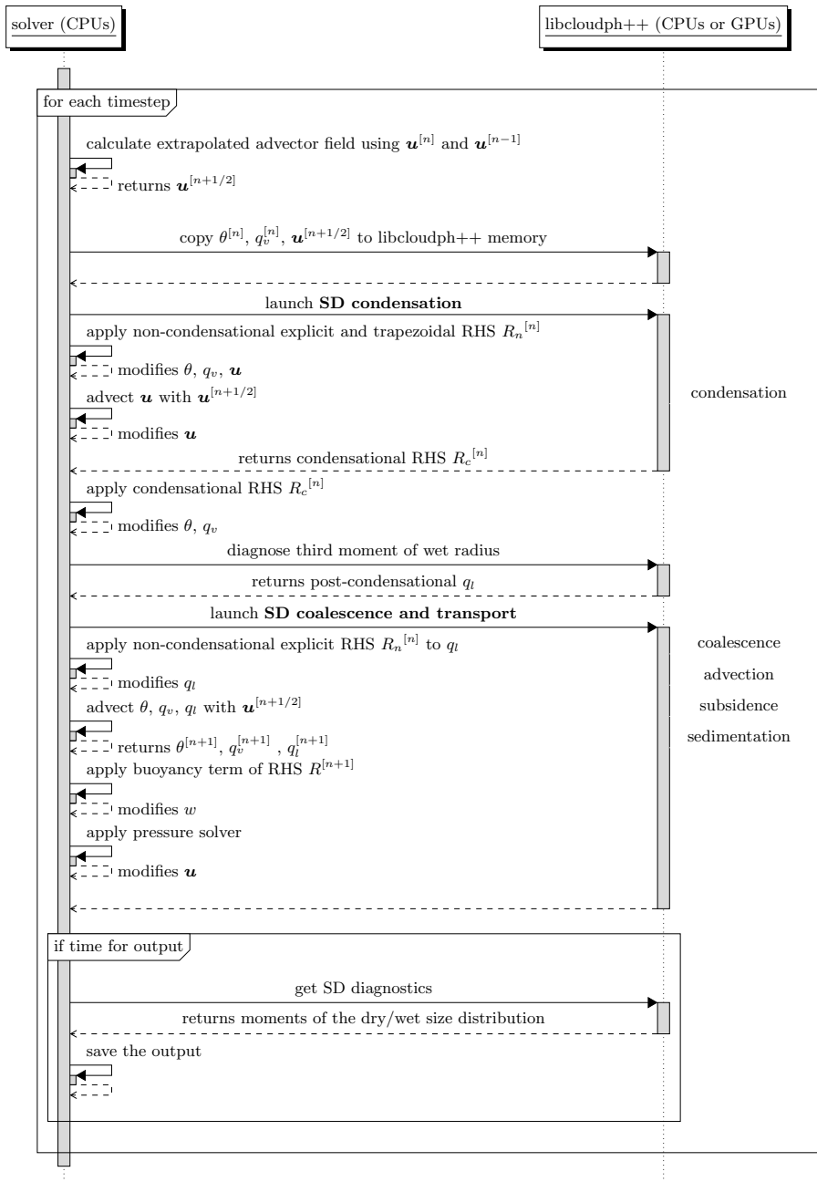
Figure 1. UML sequence diagram showing the order of operations within a single time step. Calls in boldface start microphysical calculations that are done on GPUs simultaneously with solver operations done on CPUs. The RHS is divided into condensational and non-condensational parts, R = R_n + R_c .
