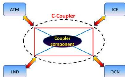
Figure 1—General architecture of models coupled with C-Coupler. “ATM” means an atmosphere model, “OCN” means an ocean model, “ICE” means a sea ice model and “LND” means a land surface model. (from Liu et al., 2014).
