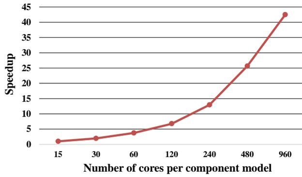
**Figure 17** **Figure 16** The parallel speedup of dynamic 3-D coupling (for 100 ping-pong couplings) between the two component models, with a new configuration derived from the configuration used in **Fig. 12** **Fig. 11**. The speedup is normalized to the time at 15 cores per component model (1583 s).
