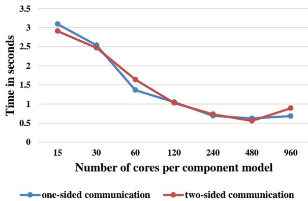
[Figure 13](#)[Figure 12](#) Comparison of data transfer times (for 100 ping-pong couplings) between a one-sided and a two-sided implementation, with the same configuration as [Fig. 12](#)[Fig. 11](#).
