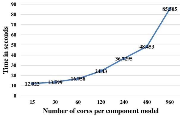
**Figure 12** **Figure 11** Initialization cost for coupling two toy models with C-Coupler2 on a supercomputer with Intel Xeon CPUs and an InfiniBand network.
