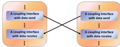
Figure 4Figure 3 Example of model coupling between two component models: deadlocks occur when blocking data send/receive operations are used.
