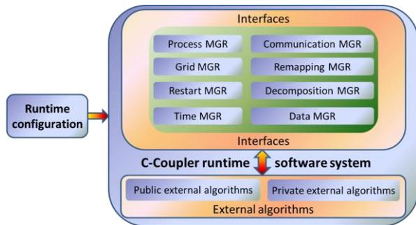
Figure 3 Figure 2 C-Coupler1 software structure.
