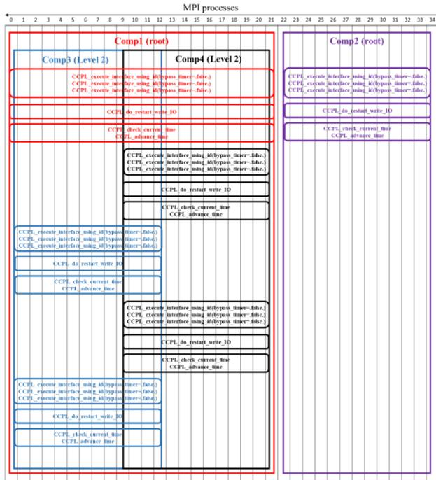
**Figure 8** **Figure 7** An example of model coupling in the kernel (time integration) stage of a coupled model constructed with C-Coupler2. *Comp1–comp4* are the four component models. Labels and boxes of the same color correspond to the same component model.
