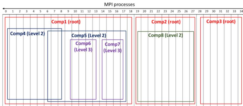
Figure 5 Sample process layout of component models (comp1–comp8).
