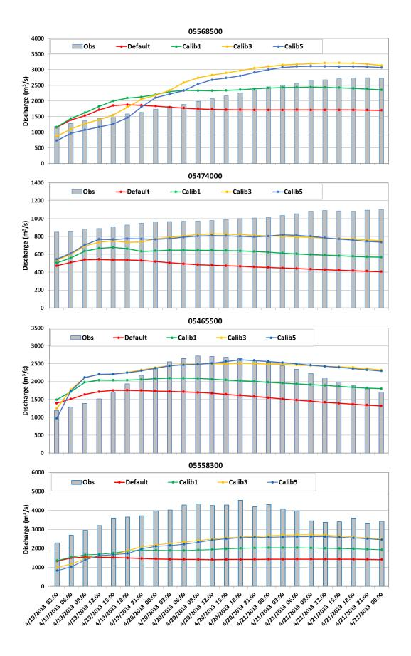
Figure S2: Observed and modeled discharge (m³/sec) using default and calibrated parameters during a 3-day calibration period (April 19–21, 2013) over four local stations. Station numbers are indicated on top of each panel.
