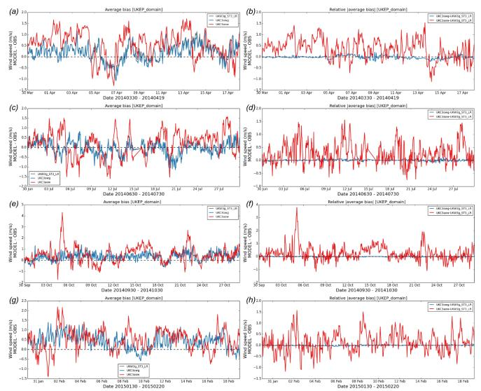
Figure 6: Difference of wind forcing applied to wave model. (a,c,e,g) Time series of average MODEL – OBSERVATION bias across all observing sites for each simulation for July 2014, April 2014, October 2014 and Feburary 2015 respectively. (b,d,f,h) Differences in absolute | MODEL – OBS | bias for each simulation period relative to the UKW3g wind forcing.
