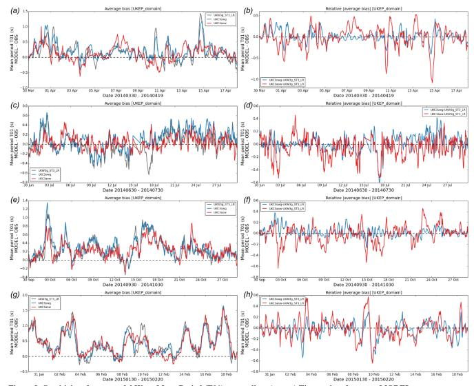
Figure 8: Sensitivity of wave model Wave Mean Period (T01) to coupling. (a,c,e,g) Time series of average MODEL – OBSERVATION bias across all observing sites for each simulation for July 2014, April 2014, October 2014 and Feburary 2015 respectively. (b,d,f,h) Differences in absolute | MODEL - OBS | bias for each simulation period relative to UKW3g.
