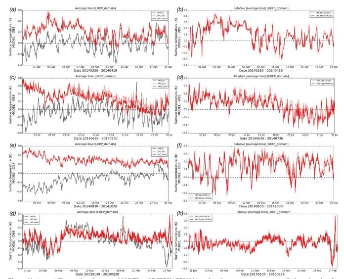
Figure 10: (a,c,e,g) Time series of average MODEL – OBSERVATION bias of surface temperature across all observing sites for each simulation for July 2014, April 2014, October 2014 and February 2015 respectively. (b,d,f,h) Differences in absolute | MODEL – OBS | bias for each simulation period relative to UKA3u. A negative relative | average bias | indicates the coupled system to have a lower average absolute bias across all observation sites than the control.
