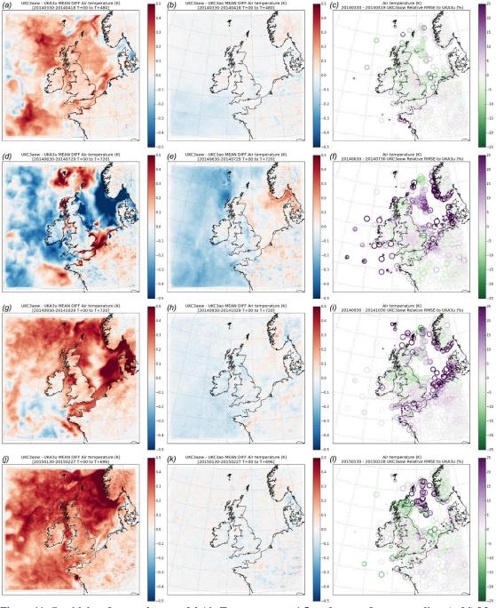
Figure 11: Sensitivity of atmosphere model Air Temperature at 1.5 m above surface to coupling. (a,d,j) Monthly mean difference between fully coupled and daily updated OSTIA [UKC3aow – UKA3u] during April, July, October 2014 and February 2015 runs respectively. (b,e,h,k) Monthly mean difference between fully coupled and partially coupled [UKC3aow – UKC3ao] runs during each experiment (c,f,i,l) Percentage difference in Air Temperature RMSE statistic for UKC3aow relative to UKA3u.
