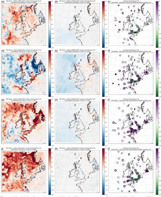
Figure 9: Sensitivity of atmosphere model Surface Temperature to coupling. (a,d,j) Monthly mean difference between fully coupled and daily updated OSTIA [UKC3aow – UKA3u] during April, July, October 2014 and February 2015 runs respectively. (b,e,h,k) Monthly mean difference between fully coupled and partially coupled [UKC3aow – UKC3ao] runs during each experiment (c,f,i,l) Percentage difference in Surface Temperature RMSE statistic for UKC3aow relative to UKA3u.
