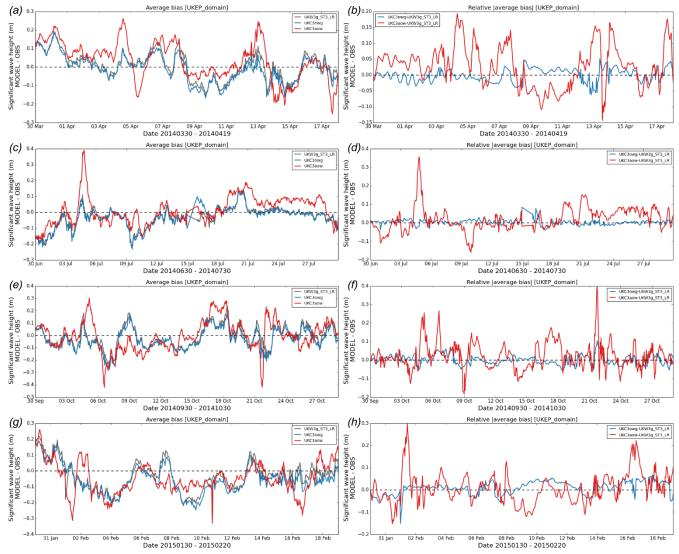
Figure 7: Sensitivity of wave model Siginificant Wave Height (Hs) to coupling. (a,c,e,g) Time series of average MODEL – OBSERVATION bias across all observing sites for each simulation for July 2014, April 2014, October 2014 and Feburary 2015 respectively. (b,d,f,h) Differences in absolute | MODEL – OBS | bias for each simulation period relative to UKW3g.
