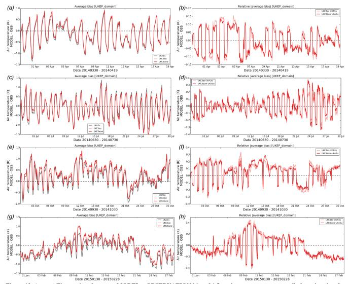
Figure 12: (a,c,e,g) Time series of average MODEL - OBSERVATION bias of 1.5 m air temperature across all observing sites for each simulation for July 2014, April 2014, October 2014 and Feburary 2015 respectively. (b,d,f,h) Differences in absolute | MODEL - OBS | bias for each simulation period relative to UKA3u. A negative relative |average bias| indicates the coupled system to have a lower average absolute bias across all observation sites than the control.
