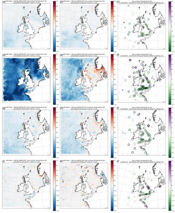
Figure 3: Sensitivity of ocean model Sea Surface Temperature to coupling. (a,d,j) Monthly mean difference between fully coupled and ocean only [UKC3aow – UKO3g] during April, July, October 2014 and February 2015 runs respectively. (b,e,h,k) Monthly mean difference between fully coupled and partially coupled [UKC3aow – UKC3ao] runs during each experiment. Note the different colour scale. (c,f,i,l) Percentage difference in Surface Temperature RMSE statistic for UKC3aow relative to UKO3g.
