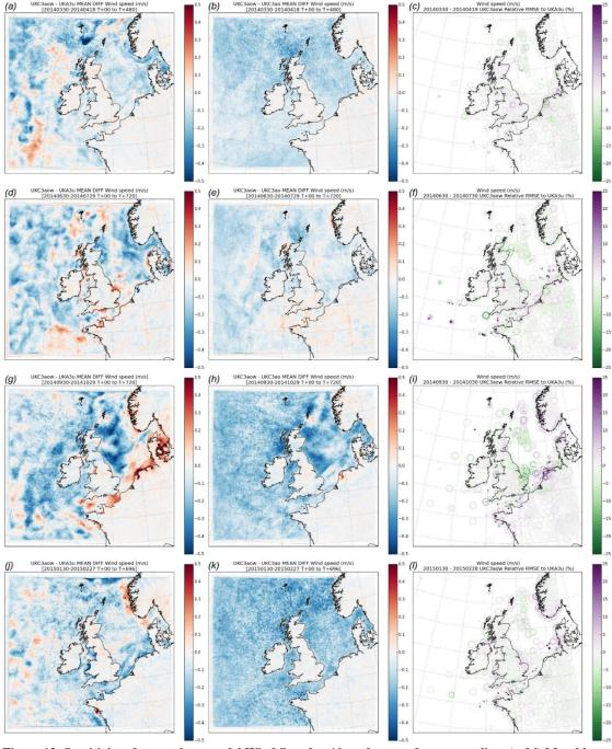
Figure 13: Sensitivity of atmosphere model Wind Speed at 10 m above surface to coupling. (a,d,j) Monthly mean difference between fully coupled and daily updated OSTIA [UKC3aow – UKA3u] during April, July, October 2014 and February 2015 runs respectively. (b,e,h,k) Monthly mean difference between fully coupled and partially coupled [UKC3aow – UKC3ao] runs during each experiment (c,f,i,l) Percentage difference in wind speed RMSE statistic for UKC3aow relative to UKA3u.
