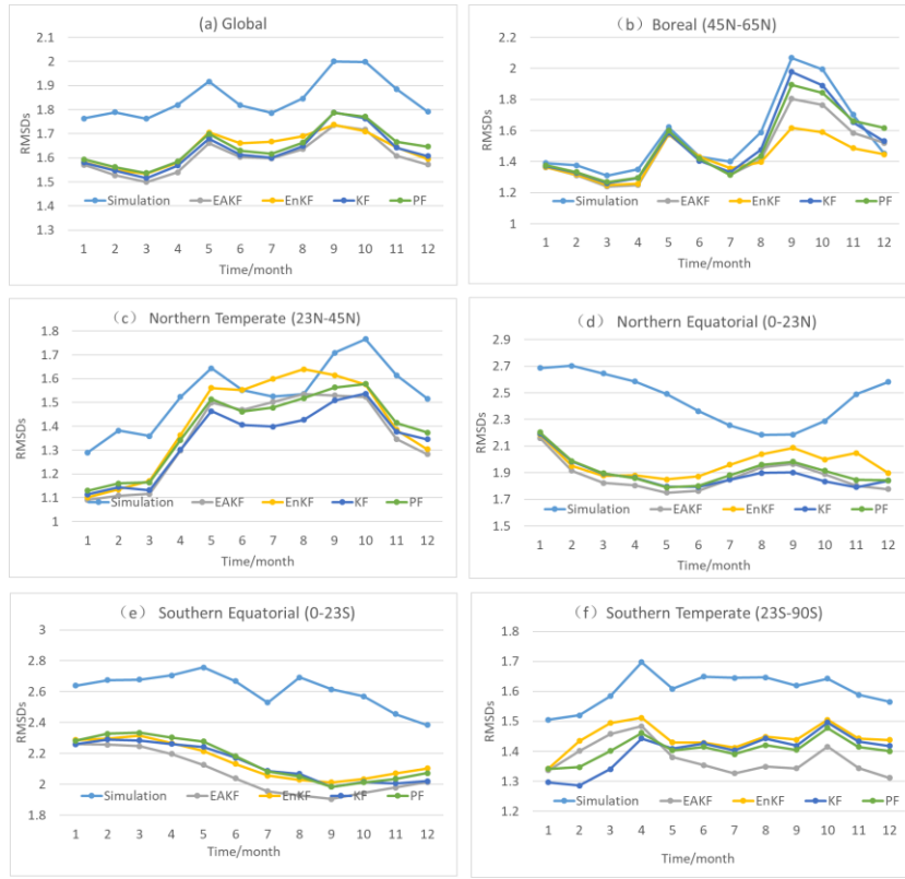
Figure 4: RMSDs of ensemble means of simulation/assimilation versus GEOV2 LAI for (a) global, (b) boreal (45-65°N), (c) northern temperate (23-45°N), (d) northern equatorial (0-23°N), (e) southern equatorial (0-23°S), and (f) southern temperate (23-90°S).
