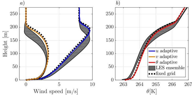
**Figure 4.** Time averaged profiles over the eight hour of the run according to the GABLS1 intercomparison scenario. For (a) the horizontal wind components and (b) the potential temperature. Results are obtained with the present adaptive-grid SCM (coloured lines), the LES models ensemble (i.e mean  $\pm \sigma$ ) from Beare et al. (2006) (grey-shaded areas) and the present SCM, employing an equidistant and static grid with a 6.25 meter resolution (dashed lines).
