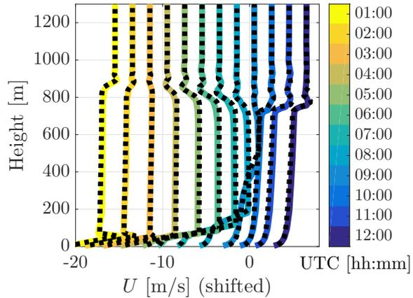
**Figure 7.** Vertical profiles of the wind-speed magnitude  $U$  obtained with the adaptive-grid (in colour) and the fixed equidistant-grid (dashed) SCMs. The twelve plotted profiles are obtained for the 24-th of October with an hourly interval, starting from 1:00 AM local time. Noting that the profiles are shifted in order to distinguish between the different times (with vanishing wind at the surface).
