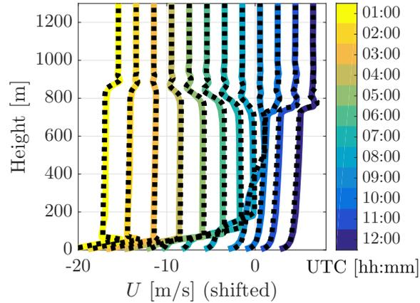
**Figure 7.** Vertical profiles of the wind-speed magnitude  $U$  obtained with the adaptive-grid (in colour) and the fixed equidistant-grid (dashed) SCMs. The twelve plotted profiles are obtained for the [23-th](#)–[24-th](#) of October with an hourly interval, starting from 1:00 AM local time. Noting that the profiles are shifted in order to distinguish between the different times (with vanishing wind at the surface).
