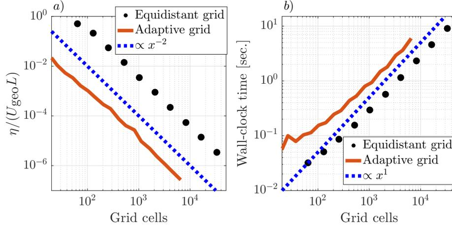
**Figure 3.** The scaling characteristics for the laminar-Ekman-spiral case. (a) Presents the error convergence for the equidistant-grid and adaptive-grid approach. The errors ( $\eta$ ) follow the slope of the blue dashed line that indicates the second-order accuracy of the methods. The wall-clock time for the different runs is presented in (b), showing that for both of the aforementioned approaches, the required effort scales linearly with the number of grid cells.
