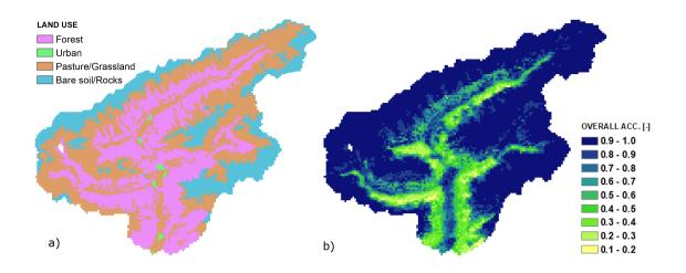
Figure 6. Pixel a) Land use distribution for the catchment and b) pixel based overall accuracy (OA) of the comparison between simulated and MODIS-derived snow cover maps, computed from January 1 to June 30, 2011 for a total of 50 MODIS snow cover maps.
