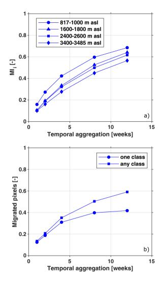
**Figure 3.** a) Band migration index for the five temporal aggregations, reported for four elevation bands (lowest elevation band from 817 to 1000 m); from 1600 to 1800 m; from 2400 to 2600 m; highest elevation band from 3400 to 3485 m). b) Fraction of migrated pixels computed for the five temporal aggregations over all the elevation bands. Circles refers to pixels that migrated of  $\pm 1$  energy class, squares to total migrated pixels.
