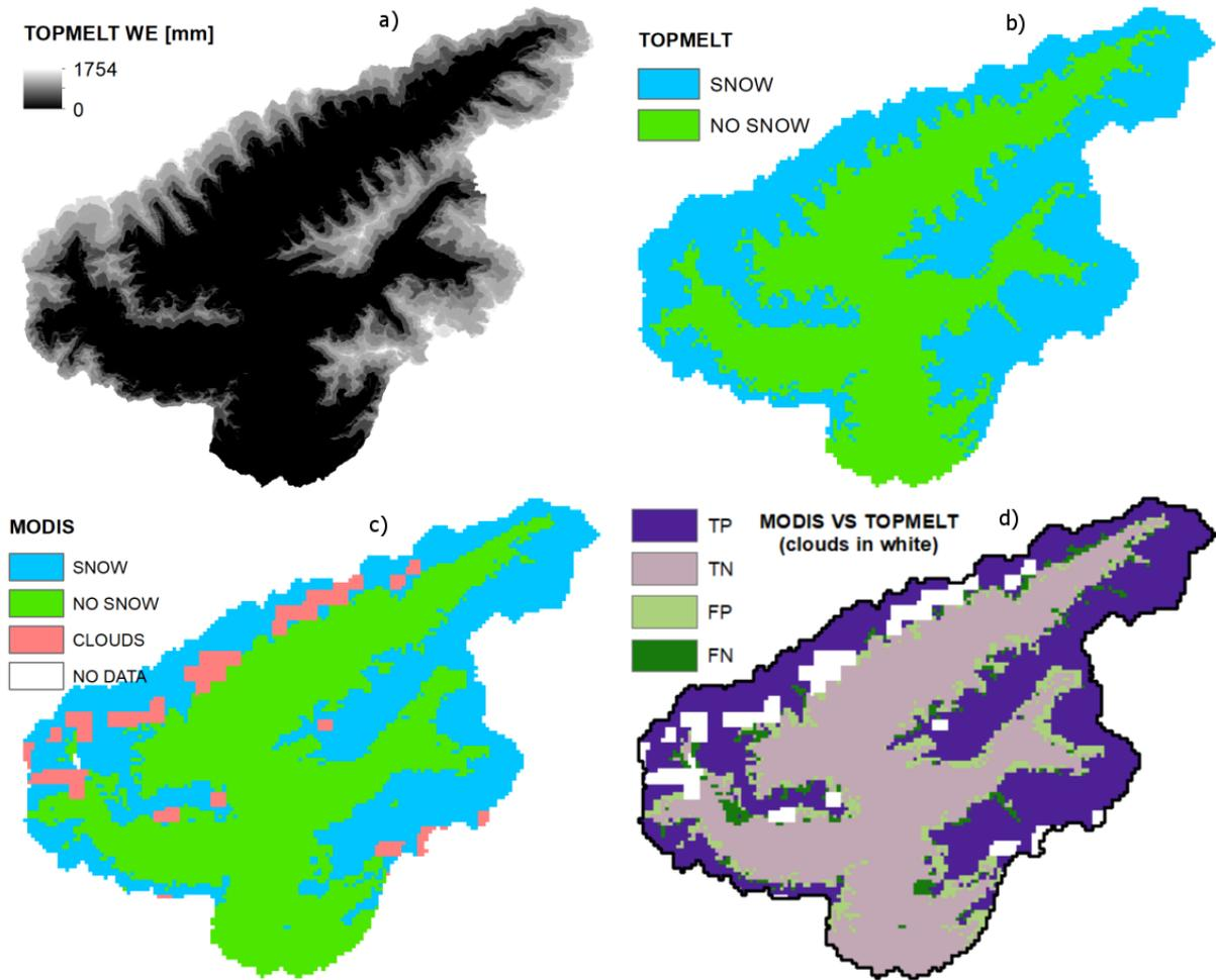
**Figure 4.** Comparison between simulated and MODIS-derived snow cover map. The comparison is obtained by using the model set up W4-C10 for May 6, 2011. TP and TN are true positives and true negatives: both TOPMELT and MODIS are indicating the presence or absence of snow at the pixel, respectively. Similarly FP and FN are false positives and false negatives.
