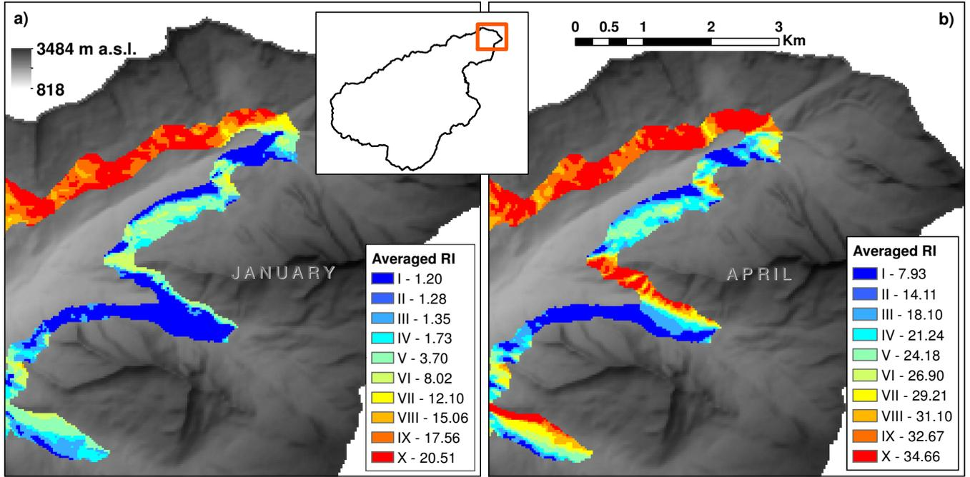
**Figure 1.** Comparison between radiation index distribution over the 2000-2200 m elevation band of the Aurino basin for a) January 1st and b) April 1st (ten classes subdivision). The figures show the north-eastern portion of the basin and report the average radiation index [ $\text{J m}^{-2} \text{h}^{-1}$ ], with the corresponding radiation class identified by a roman number.
