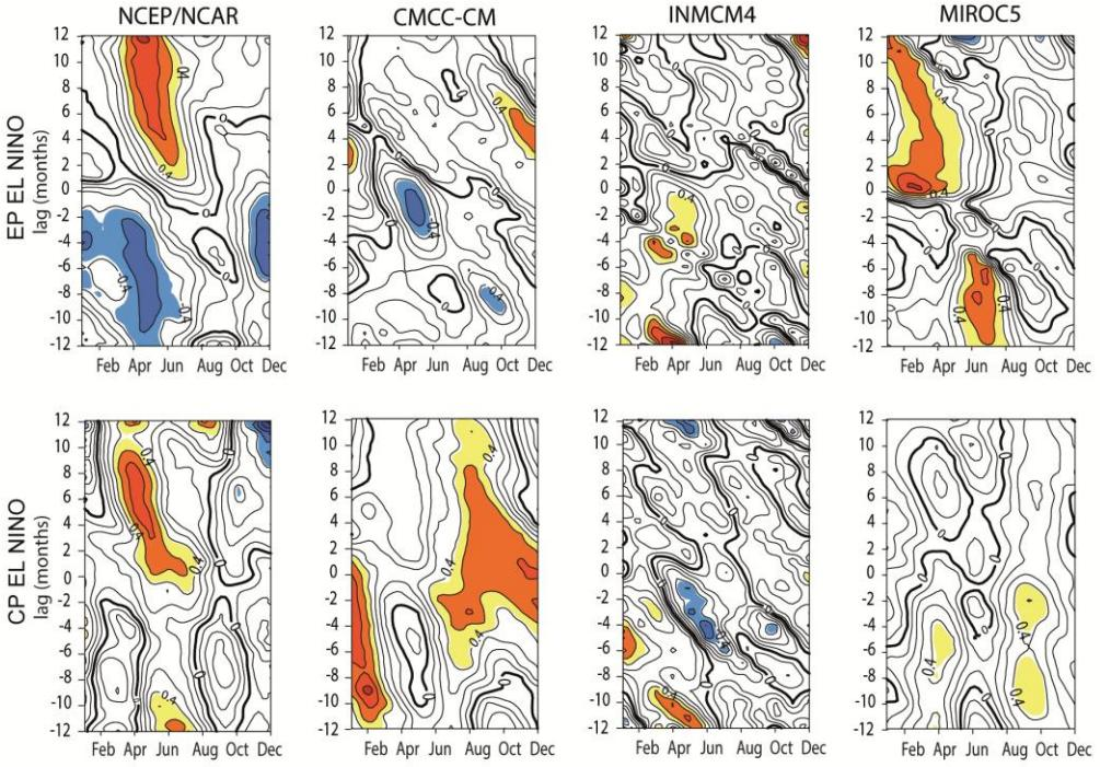
**Figure A5:** Monthly lagged correlation of E (a-d) and C (e-h) indices as a function of start month with respect to MJO activity index WPacMJOu850 for NCEP/NCAR Reanalysis and 3 CMIP5 models. Contour interval is 0.1. Negative correlation  $\leq -0.42$  is blue shaded, positive correlation  $\geq 0.42$  is orange shaded (90% significance level).
