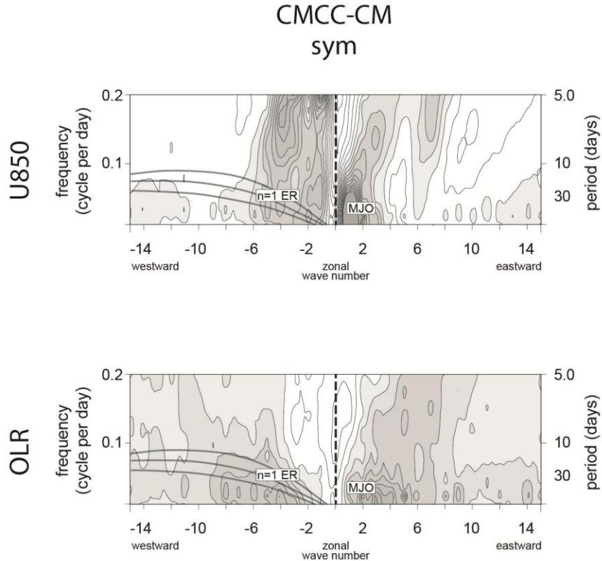
**Figure C1:** Space–time spectrum of the 15°N–15°S symmetric component of U850 (upper panel) and OLR (bottom panel) divided by the background spectrum for CMCC-CM model
