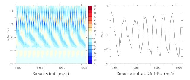
**Figure 1.** Left panel: Altitude-time profile of the zonal wind (in m s $^{-1}$ ), averaged between 10 $^{\circ}$  S and 10 $^{\circ}$  N, from a simulation with evolving background aerosol. The vertical axis shows the logarithm of the pressure in Pa. Right panel: Zonal wind at 25 hPa, averaged between 10 $^{\circ}$  S and 10 $^{\circ}$  N.
