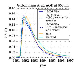
**Figure 7.** Same as Fig. 6, but here the dashed (resp. dotted) line shows the model result for SO<sub>2</sub> lifetimes uniformly doubled (resp. SO<sub>2</sub> lifetimes doubled on the day of the eruption, and decreasing linearly to their climatological values within 1 month).
