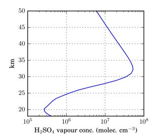
Figure 2. Simulated vertical profile of  $H_2SO_4$  number concentration at  $43^{\circ}N$  in September and October under background conditions. To be compared to measurements by Arnold et al. shown in Fig. 5c of English et al. (2011).
