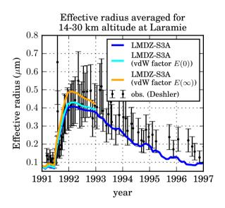
Figure 13. Stratospheric effective particle radius at Laramie, Wyoming (41° N, 105° W) as simulated by the LMDZ-S3A model and observed with optical particle counters (Deshler et al., 2003). The light blue (resp. orange) line shows the model result for coagulation enhanced by the continuum regime van der Waals enhancement factor E(0) (resp. the kinetic regime enhancement factor  $E(\infty)$ ).
