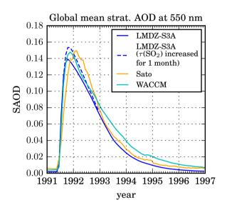
**Figure 15.** Same as Fig. 14, but here the dashed line shows the model result for an SO<sub>2</sub> lifetime doubled on the day of the eruption, decreasing linearly to climatological values within one month.
