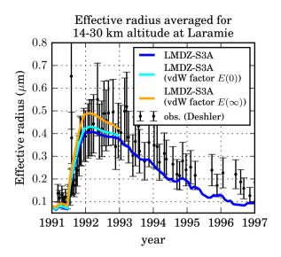
Figure 5. Stratospheric effective particle radius at Laramie, Wyoming (41° N, 105° W) as simulated by the LMDZ-S3A model and observed with optical particle counters (Deshler et al., 2003). The light blue (resp. orange) line shows the model result for coagulation enhanced by the continuum regime enhancement factor E(0) (resp. the kinetic regime enhancement factor  $E(\infty)$ ).
