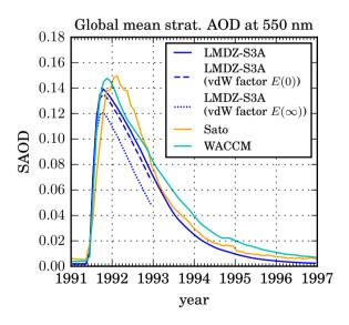
Figure 6. Evolution of the global mean stratospheric aerosol optical depth (SAOD) at 550 nm modelled with LMDZ-S3A compared to the climatology from Sato (2012) and to SAOD simulated with WACCM by Mills et al. (2016). The dashed (resp. dotted) line shows the model result for coagulation enhanced by the continuum regime enhancement factor E(0) (resp. the kinetic regime enhancement factor  $E(\infty)$ ).
