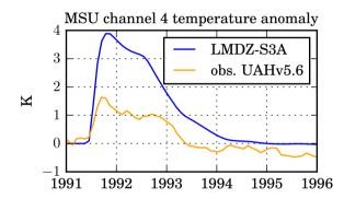
**Figure 12.** Global mean MSU channel 4 (upper tropospheric and lower stratospheric) temperature anomaly. The modelled anomaly due to the Pinatubo sulfate aerosol is computed as the difference between simulations with and without volcanic aerosol, while the observed anomaly reported by the UAH (Spencer and Christy, 1993) is with respect to the 1981–2010 base period.
