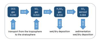
**Figure 6.** Modelled annual mean stratospheric burden (in TgS) and fluxes (in  $TgSyr^{-1}$ ) of the represented sulfur species. The values are given for steady state background conditions without any stratospheric volcanic emissions. Advection can take the species out of the stratosphere into the troposphere, where they can be removed by wet and dry deposition.
