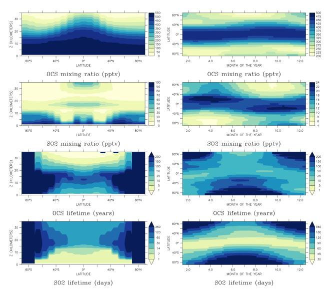
**Figure 2.** Climatological volume mixing ratios (upper half, in pptv) and lifetimes (lower half, in years or days) of OCS and SO<sub>2</sub> produced by the UPMC/Cambridge model and used as initial and boundary conditions for the LMDZ-S3A model. The left column shows the zonal and annual mean latitude-height distribution, while the right column shows an annual cycle of the zonal mean value at 20 km altitude.
