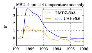
**Figure 3.** Global mean MSU channel 4 (upper tropospheric and lower stratospheric) temperature anomaly. The modelled anomaly due to the Pinatubo sulfate aerosol is computed as the difference between simulations with and without volcanic aerosol, while the observed anomaly reported by the UAH (Spencer and Christy, 1993) is with respect to the 1981–2010 base period.
