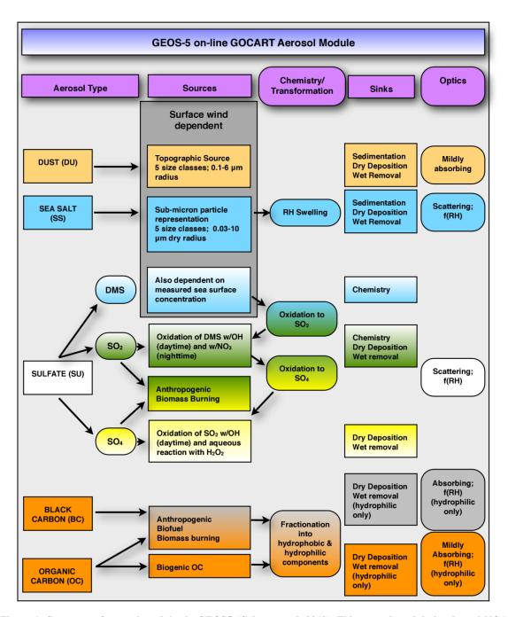
Figure 1: Summary of aerosol modules in GEOS5 (Colarco et al. 2010). This aerosol module is adopted NGACv2. (Provided by Colarco).
