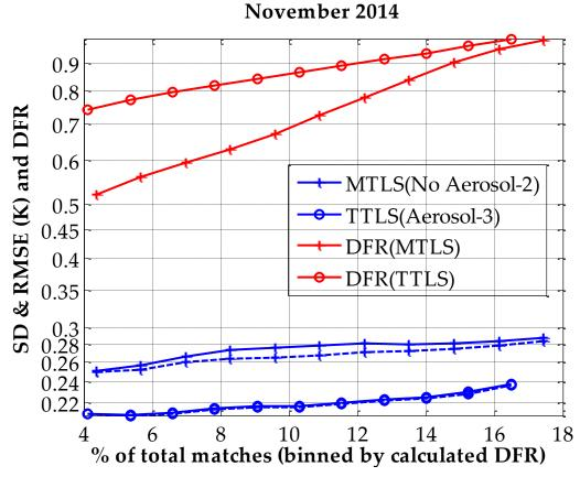
Figure 5: Comparison of retrieval accuracy (blue lines) and algorithm sensitivity (Degrees of Freedom in Retrieval, red lines) of MTLS (plus) without aerosol and Truncated Total Least Squares (solid circles) using aerosol optical depth in the state vector for MODIS-Aqua data for January 2015. Evaluation is done against *i*Quam buoy data
