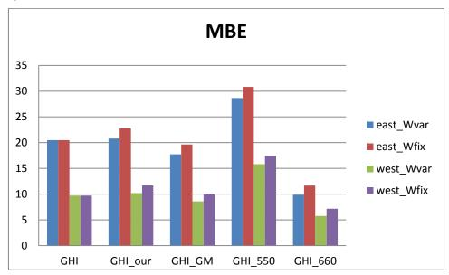
5 Figure 6: a) Aerosol impact on DNI from Perez model estimations; b) NGACv2 AOD impact on Perez model solar energy estimation an bias error (MSE); east- GOES eastern USA satellite; west – GOES western USA; Wvar – variable water vapor (GFS model); Wfix monthly averaged water vapor (NASA); "our" – monthly averaged AOD used in ASRC (NASA); "GM" – Gueymard AOD; "550" and "660" - NGACv2 AOD.
