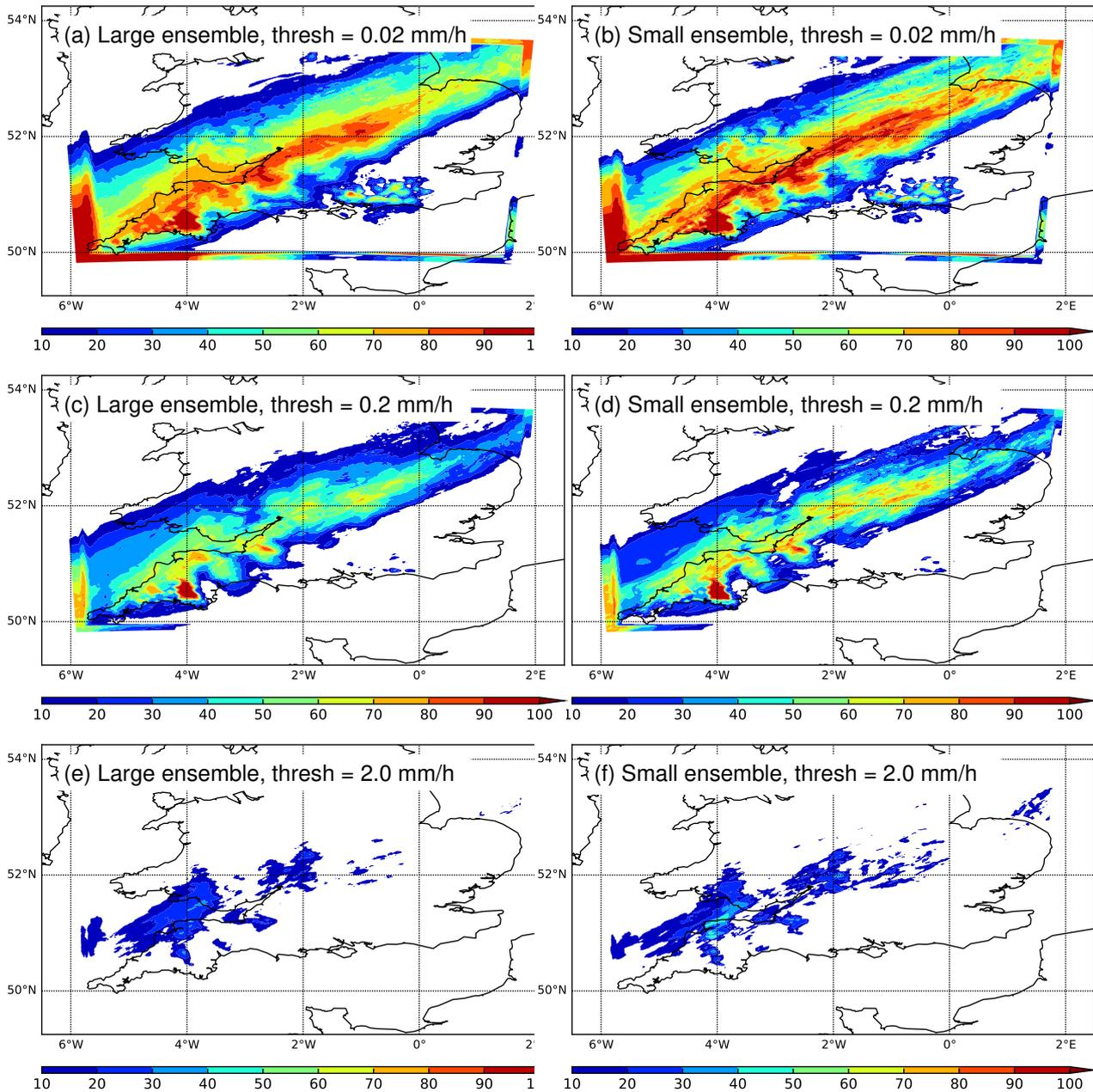
**Figure 8.** Probability of rain for 20th September 2011 15Z based on the percentage of ensemble members that forecast rain in each grid box above thresholds of  $>0.02$  mm/h (top row),  $>0.2$  mm/h (middle row), and  $>2.0$  mm/h (bottom row). Plots are for the large (left column) and the small (right) ensemble. The intermediate and small ensembles each represents a single sample from the large ensemble.
