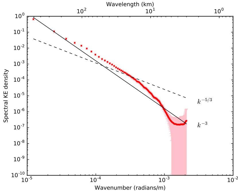
**Figure 9.** The large ensemble’s mean kinetic energy spectrum  $\bar{E}^{(93)}(k)$  (red dots), the sample standard deviation (red error bars), and the  $k^{-5/3}$  and  $k^{-3}$  lines for comparison. See the text for a description of how the kinetic energy spectrum is computed.
