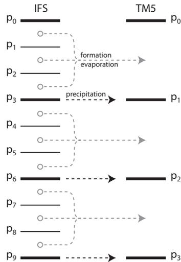
**Figure 1.** Regridding of additional meteorological fields in the coupling process between IFS and TM5. The mass flux of falling precipitation is directly sampled at the pressure levels shared by both modules. For precipitation formation and evaporation a volume-weighted average is calculated for multiple IFS pressure levels corresponding to one TM5 pressure level.
