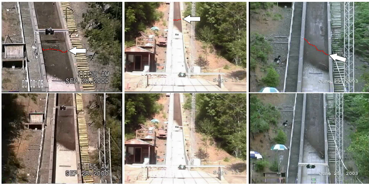
Figure 10. Snapshots of the flow front of test 000928 (left) 5.6 s after release (bottom left) when the approaching second surge (top left) unified with the front. The same happened in test 010913 (center top and center bottom) 7.4 seconds after release and in test 030625 (right top and right bottom) 7.0 seconds after release. The upper row of images capture the moment about half a second earlier in time than the lower row, showing the approaching second surge (indicated by the white arrows and a red line, the surge is more apparent in the video, see Logan and Iverson (2013)). In the lower row, the moments are shown were the second surge reaches the flow front. The corresponding time coincided with a sudden increase in front velocity; see Fig. 9.
