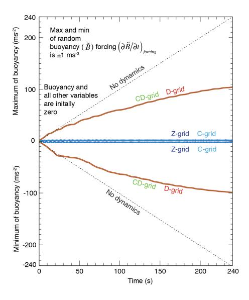
Figure 14: Time change of the maxima and minima of buoyancy ( $\hat{B}$ ) for the Z-, C-, D-, and DC-grid simulations in the presence of noisy heating patterns. The thin dashed line indicates the time change when the response of vorticity and divergence is turned off.
