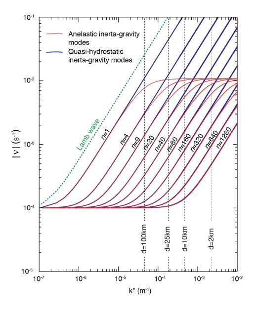
**Figure 15:** Plots of the absolute value of frequency for inertia-gravity modes obtained with the anelastic (red curves) and the quasi-hydrostatic (black curves) systems. The frequency of Lamb wave with the quasi-hydrostatic system is indicated with the dashed green curves.
