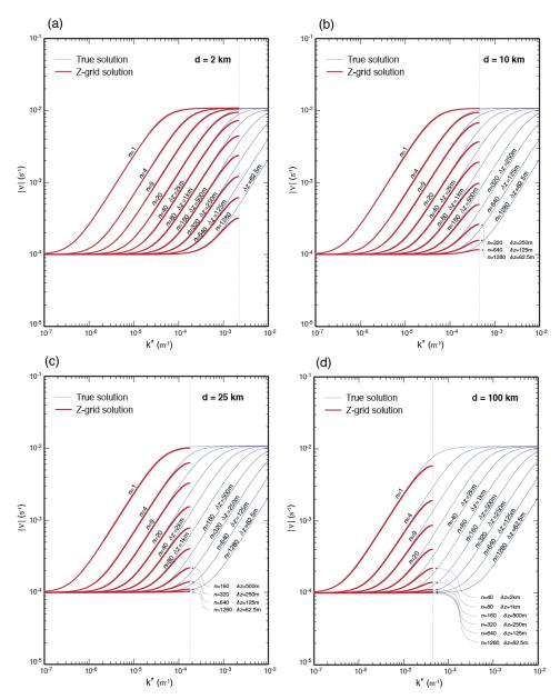
**Figure 2:** Plots of the absolute value of frequency obtained on the Z grid (red lines) for the grid spacings (a) 2 km, (b) 10 km, (c) 25 km, and (d) 100 km, and for the various vertical wave numbers. The blue thin lines are the corresponding true frequencies.
