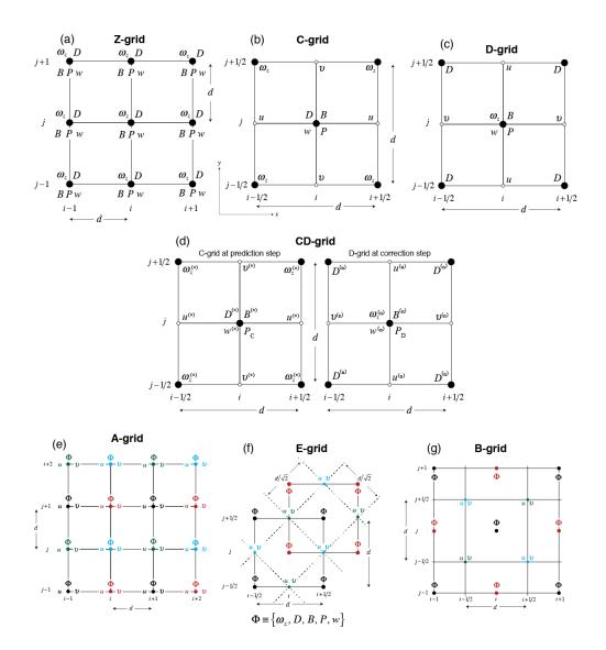
**Figure 1:** Portions of (a) the Z, (b) C, (c) D, (d) CD, (e) A, (f) E, and (g) B grids on a square grid. Colored grid points in A, E and B grids indicate the network of grid points, on which the decoupled solutions exist.
