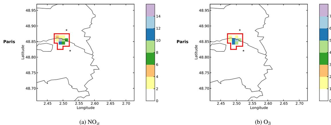
**Figure 9.** Differences between SinG and Polair3D in the surface concentrations (in % for the means over the whole simulation period) of (a)  $NO_x$  and (b)  $O_3$ . The red-boundary enclosed area corresponds to the grid cells where the street network is located. Grid cell concentrations were calculated by combining the street-network and above-roof-top concentrations weighted by the corresponding volumes. The stars show the locations of the urban background air monitoring stations.
