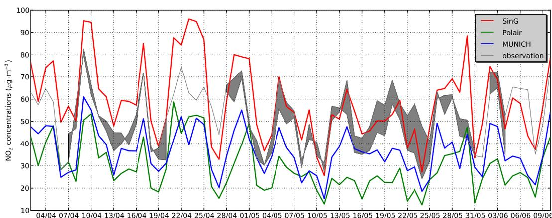
**Figure 7.** Temporal evolution of NO<sub>2</sub> daily-averaged concentrations modeled with MUNICH (blue line) and the SinG model (red line). They are compared to the measured concentrations (black shaded regions) at the stations nearby traffic on each sidewalks of the Boulevard Alsace-Lorraine. If the measurement is available only one station, black line is used instead.
