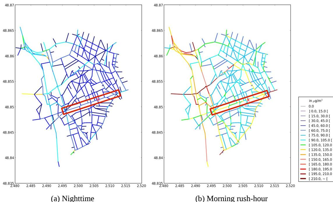
**Figure 6.** Simulated  $\text{NO}_x$  concentrations using MUNICH (a) during nighttime at 1 AM (UTC) (b) in the morning rush-hour at 7 AM (UTC) on March 25, 2014. The red rectangular box encompasses Boulevard Alsace-Lorraine and the cross mark corresponds to the location of the air monitoring stations on the sidewalks.
