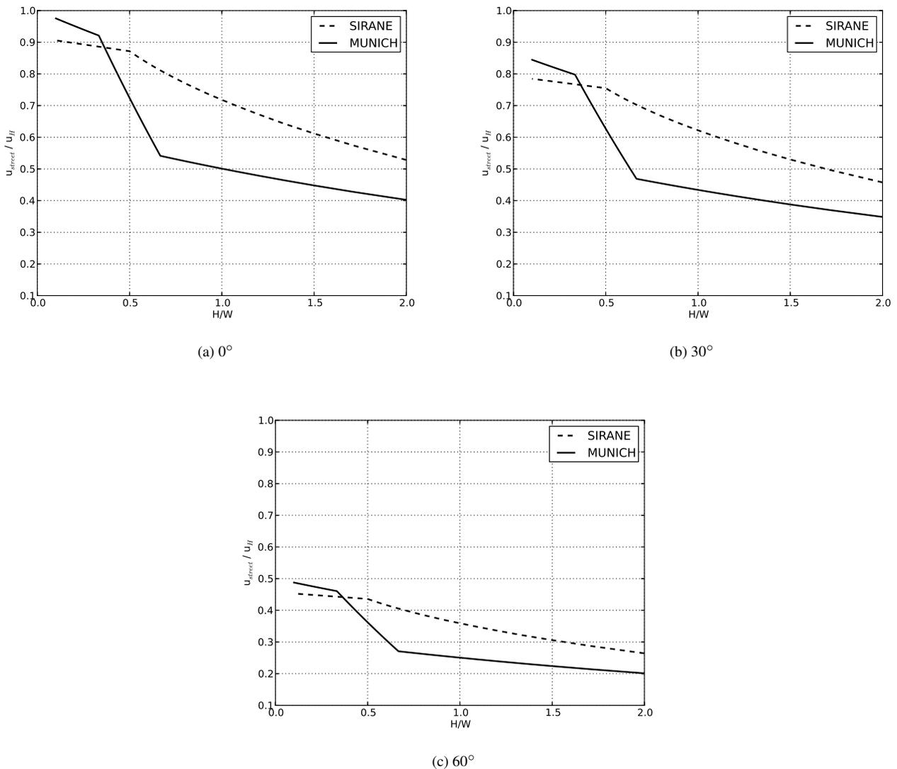
**Figure 2.** Comparison of the mean horizontal wind velocity (normalized with respect to the wind speed at roof level) within the street-canyon calculated with the profiles of SIRANE (Soulhac et al., 2008) (dotted lines) and MUNICH (Lemonsu et al., 2004) (solid lines) as a function of the street aspect ratio for three different angles between the wind direction and the street direction (a)  $0^\circ$ , (b)  $30^\circ$ , (c)  $60^\circ$
