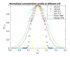
Figure 7. Dimensionless concentration distribution across the cross-section.
