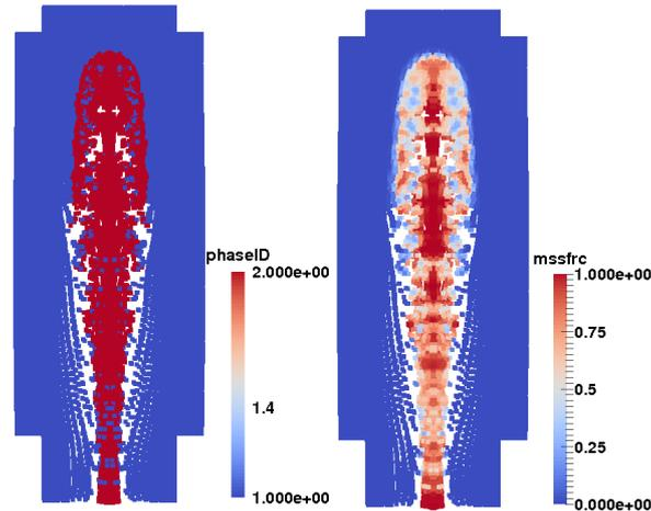
**Figure 10.** The left figure shows particle distribution. Particles of phase 1 (blue) are gradually entrained and mixed with erupted particles (red) as jet flows down stream. The right figure shows the mass fraction of erupted material at the moment corresponding to the left figure.
