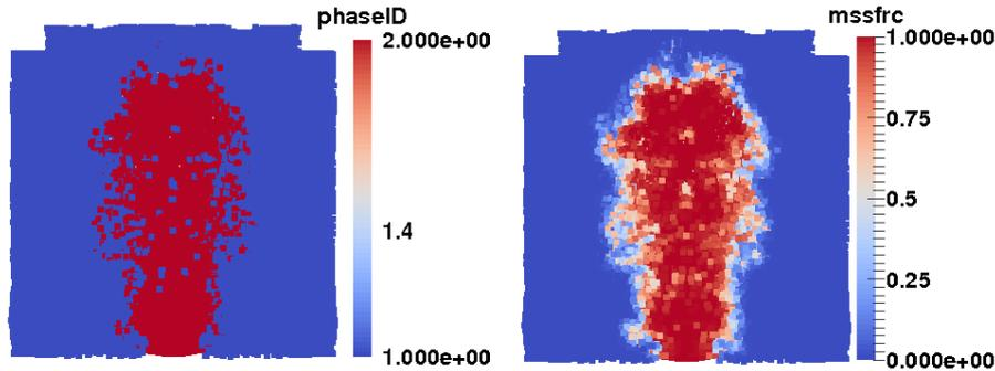
**Figure 1.** In the left figure, the blue particles (phaseID=1) represent air particles the red ones (phaseID=2) represent erupted material. The right figure shows corresponding mass fraction. Mass fraction are evaluated based on Eq. (57) and Eq. (57) without any other interface track or capture method.
