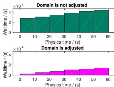
**Figure 5.** The effect of domain adjusting on simulation time. The figure on the top shows execution time without domain adjusting, the figure on the bottom shows execution time with domain adjusting. Different bins represent execution time up to specific physical time indicated by horizontal axis.
