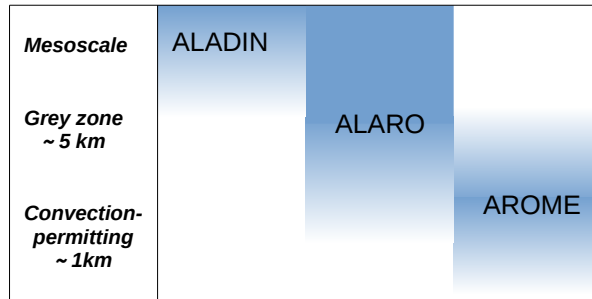
Figure 2. The different LAM configurations of the ALADIN System and their target resolutions.
