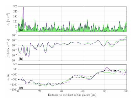
**Figure 3.** Results of the ANC algorithm (purple): (a) absolute difference between observed and model velocities, (b) estimated friction parameter and (c) estimated bedrock elevation. The green shaded area is the difference between the noisy reference velocities and the true velocities. The green solid lines are the reference values and the black dashed line is the initial guess for the bedrock elevation.
