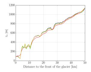
**Figure 8.** Ice surface elevation  $z_s$  after 10 years of prognostic simulation for 3 different initial states : initialisation with ATP algorithm (orange line), with ANC algorithm (purple line) and with the inversion of  $\beta$  only (red line). The green line is the reference surface elevation. The figure focuses on the first 50 km next to the front of the glacier.
