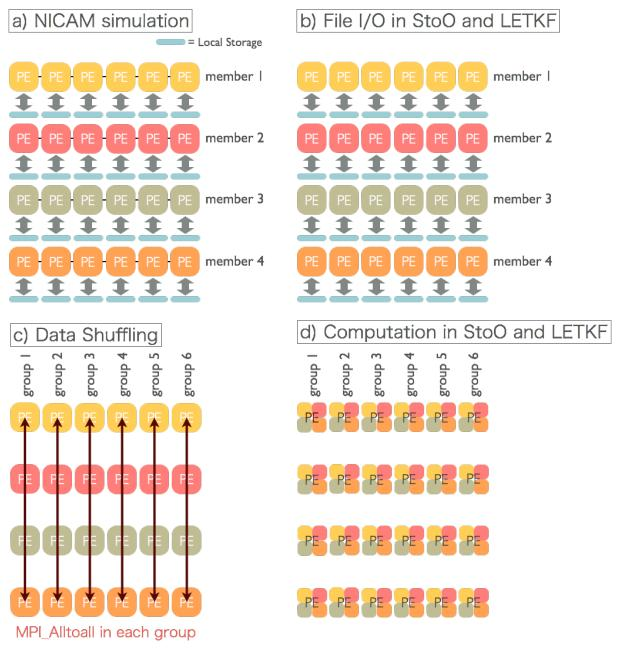
Figure 2. Schematic diagram of the proposed framework in NICAM-LETKF.
