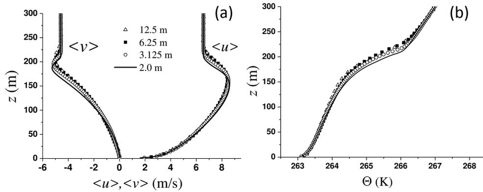
**Figure 1.** Mean wind velocity  $\langle u \rangle$  (a) and temperature  $\langle \Theta \rangle$  (b) in runs with different grid steps (spatial step is pointed in legend).
