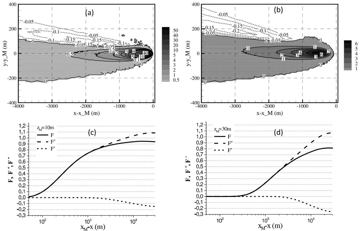
**Figure 6.** Two-dimensional footprints  $f_s(x - x_M, y - y_M, z_M)$  ( $\times 10^{-6} \text{ m}^{-2}$ ) for sensor height  $z_M = 10$  m (a) and  $z_M = 30$  m (b) and the corresponding cross-wind integrated cumulative footprints  $F(x_M - x)$  (c) and (d); long dashed line -  $F^+$  (impact of the area with positive values of  $f_s$ ); short dashed line -  $F^-$  (impact of area with negative values).
