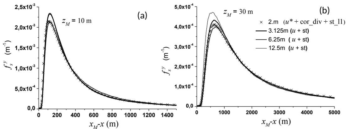
**Figure 5.** Crosswind averaged scalar flux footprints  $f_s^y$ , computed using stochastic subgrid model (28-32); (a) sensor height  $z_M = 10$  m, (b)  $z_M = 30$  m. Grid steps are given in the legend. Crosses denote footprints computed with subgrid LSM applied for the particles within the first grid layer only.
