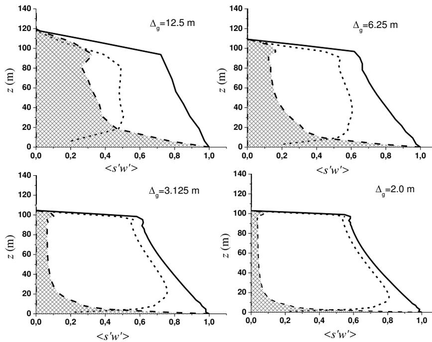
**Figure 2.** Total  $F_s^{tot} = \langle \bar{s} \bar{w} \rangle + \langle \vartheta_3^s \rangle$  (solid lines), resolved  $F_s^{res} = \langle \bar{s} \bar{w} \rangle$  (short-dashed lines) and "subgrid"  $F_s^{sbg} = \langle \vartheta_3^s \rangle$  (long-dashed lines with shading) scalar fluxes in the runs with different grid steps  $\Delta_g$ .
