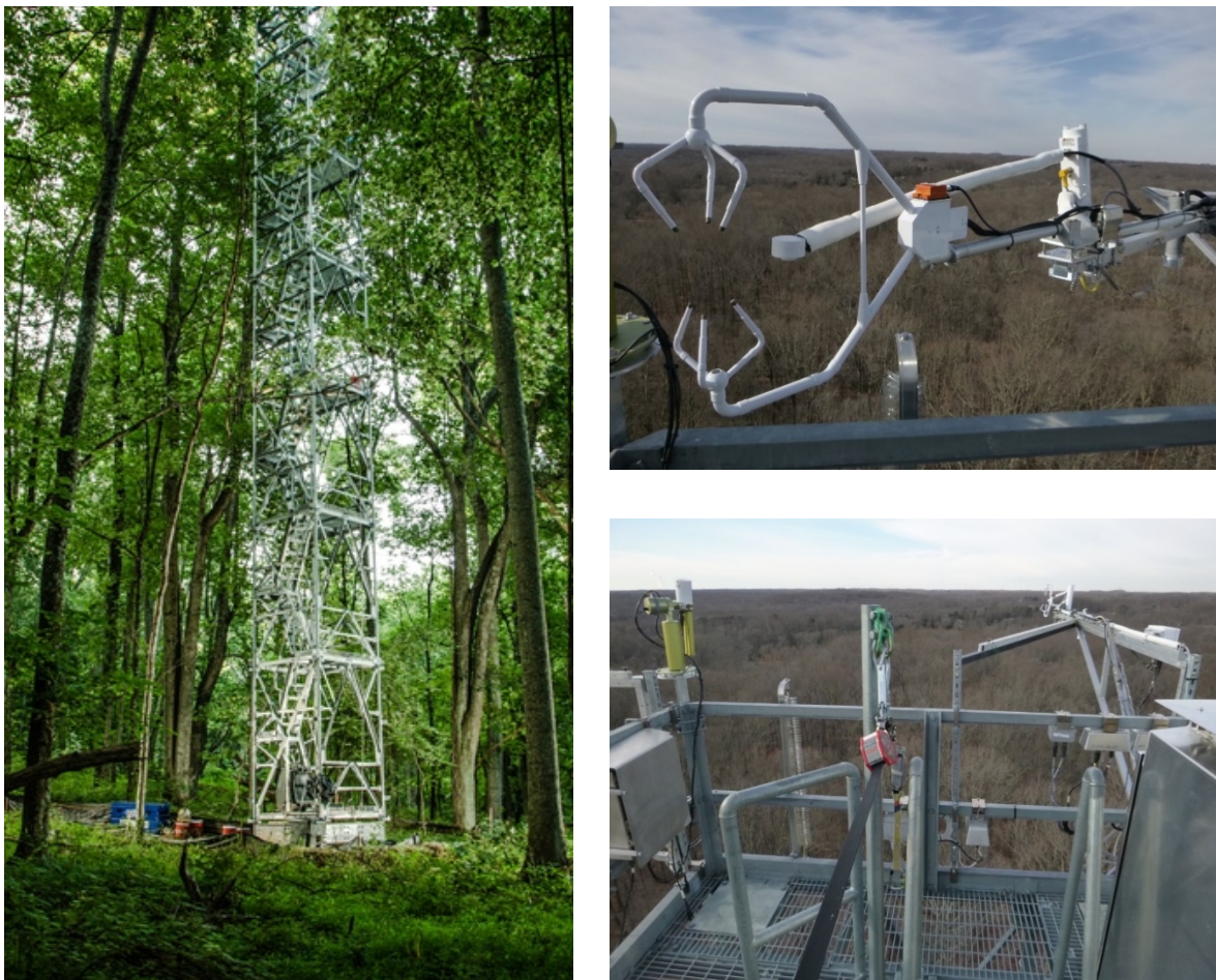
503 Figure 8. Left panel: Ecosystem at the NEON SERC tower (credit: Stephen Voss Photography; 504 http://www.stephenvoss.com/blog/neon-tower-smithsonian ). Right panels: EC instrumentation 505 on top of the NEON SERC tower. Right top panel: Campbell Scientific CSAT-3 three- 506 dimensional sonic anemometer (front) and LI-COR Biosciences LI-7200 infrared gas analyser 507 (back) on the retracted tower-top boom. Right bottom panel: Same instrumentation but with the 508 tower-top boom extended at 230° from true north.
