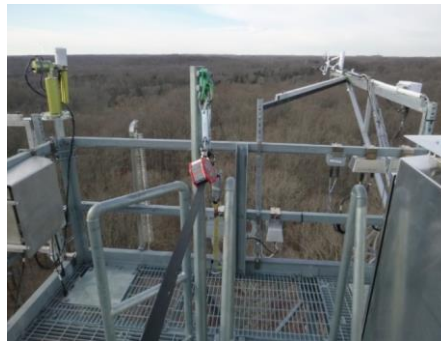
718 Figure 8. Left panel: Ecosystem at the NEON SERC tower (credit: Stephen Voss Photography; 719 http://www.stephenvoss.com/blog/neon-tower-smithsonian ). Right panels: EC instrumentation 720 on top of the NEON SERC tower. Right top panel: Campbell Scientific CSAT-3 three- 721 dimensional sonic anemometer (front) and LI-COR Biosciences LI-7200 infrared gas analyser 722 (back) on the retracted tower-top boom. Right bottom panel: Same instrumentation but with the 723 tower-top boom extended at 230° from true north.
