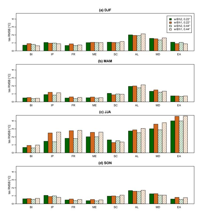
**Figure 7.** Spatial root-mean squared biases in surface air temperature by region and season with respect to the E-OBS dataset. The regions are shown in Fig. 1. Green (orange) bars are for w@h2 (w@h1), filled (hatched) bars are in comparison with E-OBS at  $0.22^{\circ}$  ( $0.44^{\circ}$ ) resolution (for w@h1, 0.22 is done by bilinear interpolation; for w@h2, 0.44 is done by aggregation).
