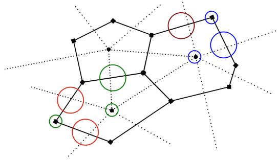
**Figure 5.** A diagram of the stencil  $EVE(v, e, i) = EC(i) \cap EV(v) - e$ . Consider the set  $(v, e, i) - (v, e, i)$  denoted in green: then  $EVE((v, e, i) - EVE(v, e, i))$  are the two red edges. Now consider the set  $(v, e, i) - (v, e, i)$  denoted in blue: then  $EVE((v, e, i) - EVE(v, e, i))$  is the brown edge.
