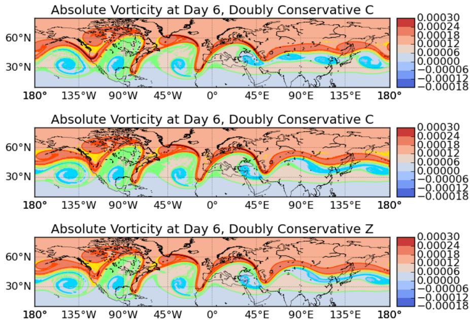
**Figure 6.** A plot of the absolute vorticity from the Galewsky et. al test case at Day 6 for the C grid scheme on a cubed-sphere grid (top panel), C grid scheme on an icosahedral grid (middle panel) and Z grid scheme on an icosahedral grid (bottom panel). The developed region of the jet is very similar for all three schemes, and is quite similar to other results in the literature. Some differences can be seen in the undeveloped region of the jet.
