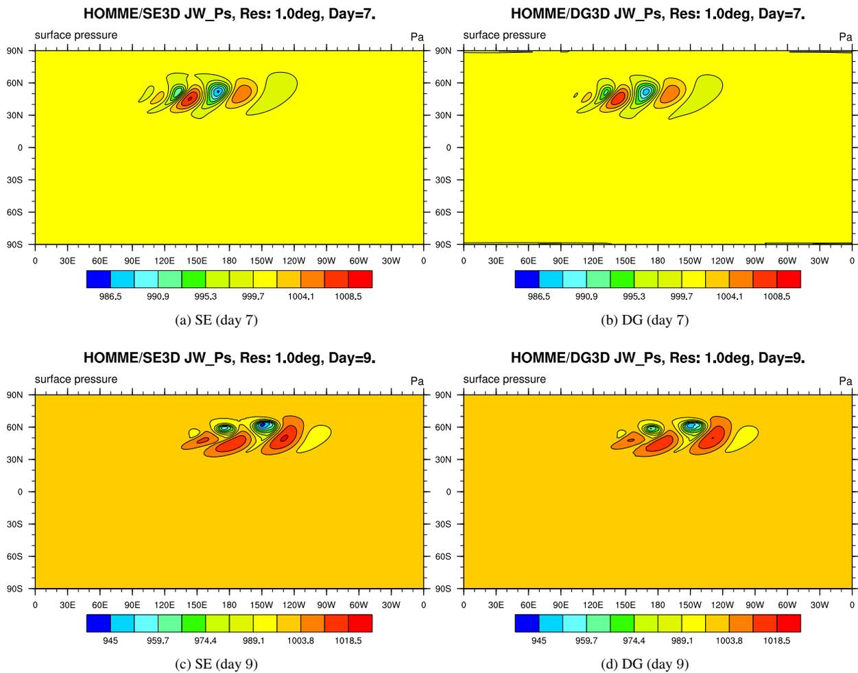
**Figure 3.** Surface pressure at day 7 and 9 for the HOMME-SE (a,c) and HOMME-DG (b,d) code for the Jablonowski-Williamson baroclinic wave instability test case. Both methods used 1 degree resolution at the equator ( $n_{lev} = 26$ , SE:  $n_p = 4$ ,  $n_e = 30$ , DG:  $n_p = 6$ ,  $n_e = 18$ ).
