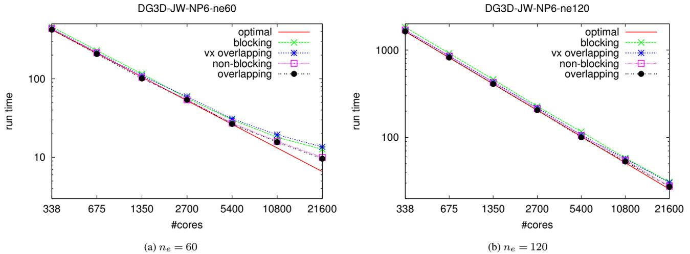
**Figure 6.** Strong scaling of the HOMME-DG code for the Jablonowski-Williamson baro-clinic wave instability test case. For the run we used  $np = 6$ ,  $nlev = 26$ , and (a)  $n_e = 60$  as well as (b)  $n_e = 120$ . For each run we compute 4500 timesteps.
