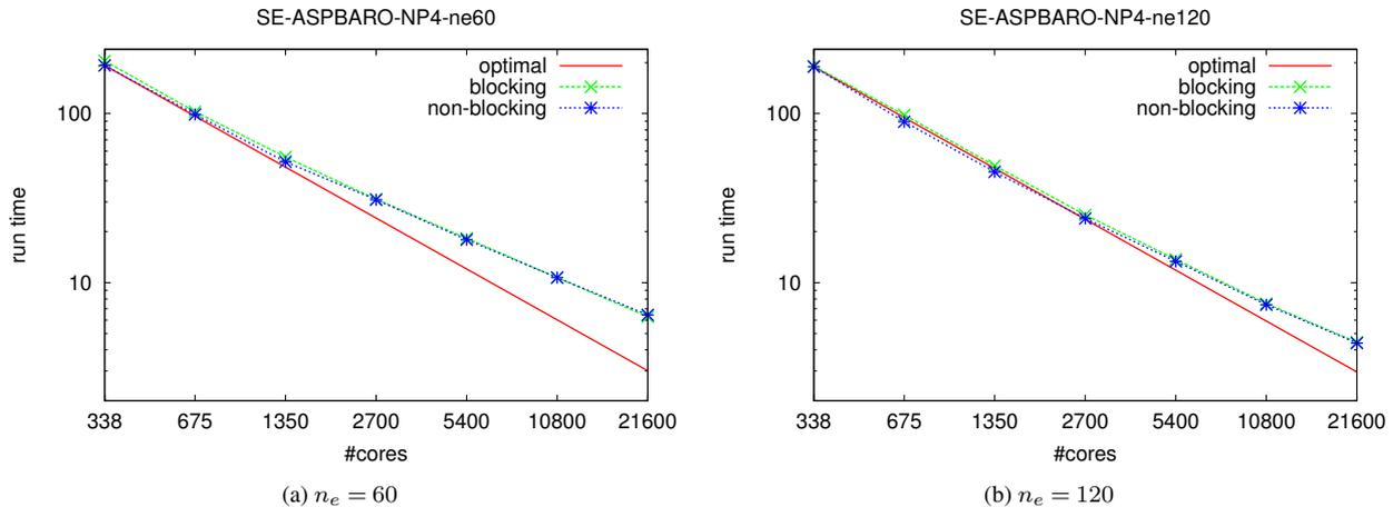
**Figure 5.** Strong scaling of the SE method in HOMME the Jablonowski-Williamson test baroclinic wave instability test case for  $n_e = 60$  (a) and  $n_e = 120$  (b). For these runs we used  $np = 4$  and  $nlev = 26$ .
