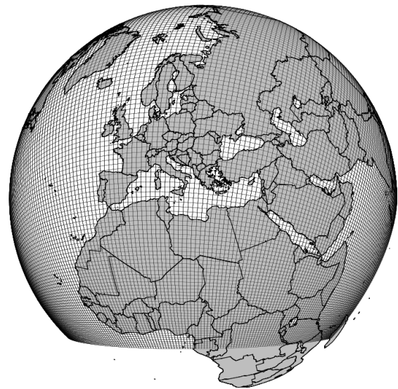
Figure 3. Model grid generated for the northern hemisphere with 180x180 points in polar stereographic projection, viewed from the top (upper panel) and from the side (lower panel).
