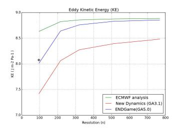
**Figure 9.** Eddy kinetic energy from sets of 12 three-day forecasts run from ECMWF analyses as a function of resolution compared to the verifying analyses reconfigured to those resolutions. Cubic interpolation of the departure point is used in the simulations shown in this plot, however the black asterisk marks GA4 at N96 with quasi-cubic interpolation.
