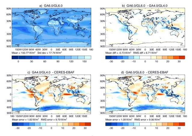
Figure 17. Top of atmosphere reflected shortwave radiation  $(Wm^{-2})$  in N96 atmosphere/land-only climate simulations of GA6.0 and GA4.0 compared with CERES EBAF (Clouds and the Earth's Radiant Energy System–Energy Balanced and Filled dataset, Loeb et al., 2009). The layout is the same as in Fig. 14.
