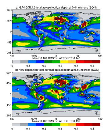
Figure 6. Mean total aerosol optical depth during SON from (a) a 10 year N96 atmosphere/land-only climate simulation using GA4.0/GL4.0 and (b) an equivalent simulation using  $z_{0,\text{CLASSIC}}/z_{0\text{m}} = 0.1$  compared to climatological values from the AERONET sun photometer network (filled squares in both plots).
