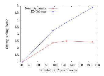
Figure 1. Strong scaling plot simulations using the ENDGame and New Dynamics dynamical cores (both using GA3.1 physics and full operational diagnostic and input/output loads) at N768 resolution on an IBM Power 7 supercomputer. Each Power 7 node contains 32 compute cores.
