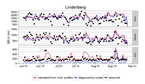
**Figure 6.** Daily minimum, mean and maximum mixing layer height as observed in Lindenberg, diagnosed by WRF-Chem and calculated from modeled profiles of temperature, wind speed and humidity (base run, 1kmx1km horizontal resolution).
