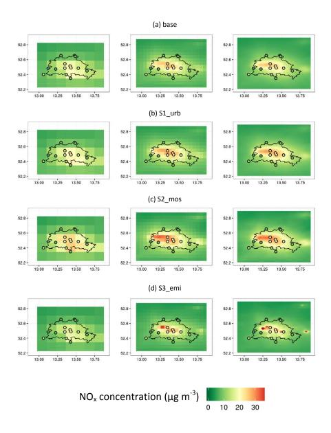
Figure 10. JJA mean modeled (colored fields) and observed (colored circles)  $NO_x$  concentration in Berlin and surroundings from a) the base run, b)  $S1_urb$ , c)  $S2_mos$ , d)  $S3_emi$ . The left column shows results obtained with the 15km horizontal resolution, the middle results from a 3km horizontal resolution and the right column shows results from a 1km horizontal resolution.
