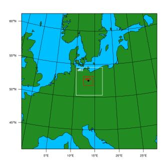
**Figure 1.** WRF-Chem model domains with horizontal resolutions of 15km (d01, outer domain), 3km (d02, middle domain) and 1km (d03, inner domain), centered around Berlin, Germany, which is marked black in the figure.
