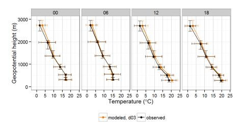
**Figure 5.** JJA mean profiles of observed and modeled (base run, 1kmx1km horizontal resolution) temperature at Lindenberg at 00:00, 06:00, 12:00 and 18:00 UTC. Error bars show the 25th and 75th percentiles of temperature and geopotential height.
