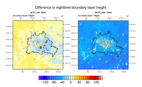
**Figure 13.** Differences in nighttime (20:00 - 02:00 UTC) mean JJA planetary boundary layer height as diagnosed from WRF-Chem, a) S1\_urb - base run, b) S2\_mos - base run (at 1km horizontal resolution).
