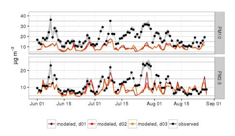
**Figure 12.** Daily mean  $PM_{10}$  and  $PM_{2.5}$  concentrations as observed and modeled (base run) at urban background stations in Berlin. Daily means are averaged over five stations for  $PM_{10}$  and four stations for  $PM_{2.5}$ . The grey shaded areas represent the variability between the different stations, showing 25th and 75th percentiles. Model results are given for all three model domains (d01 - 15km horizontal resolution, d02 - 3km, d03 - 1km).
