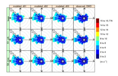
**Figure 8.** Wind roses over observed and modeled values for JJA, including observations and model results for three stations in Berlin (Tegel, Schönefeld and Tempelhof) and from all three model domains (d01 - 15km horizontal resolution, d02 - 3km, d03 - 1km). The bars refer to the frequency of how often wind was coming from the respective direction and the colors indicate how often the wind speed was observed or modeled in the indicated interval.
