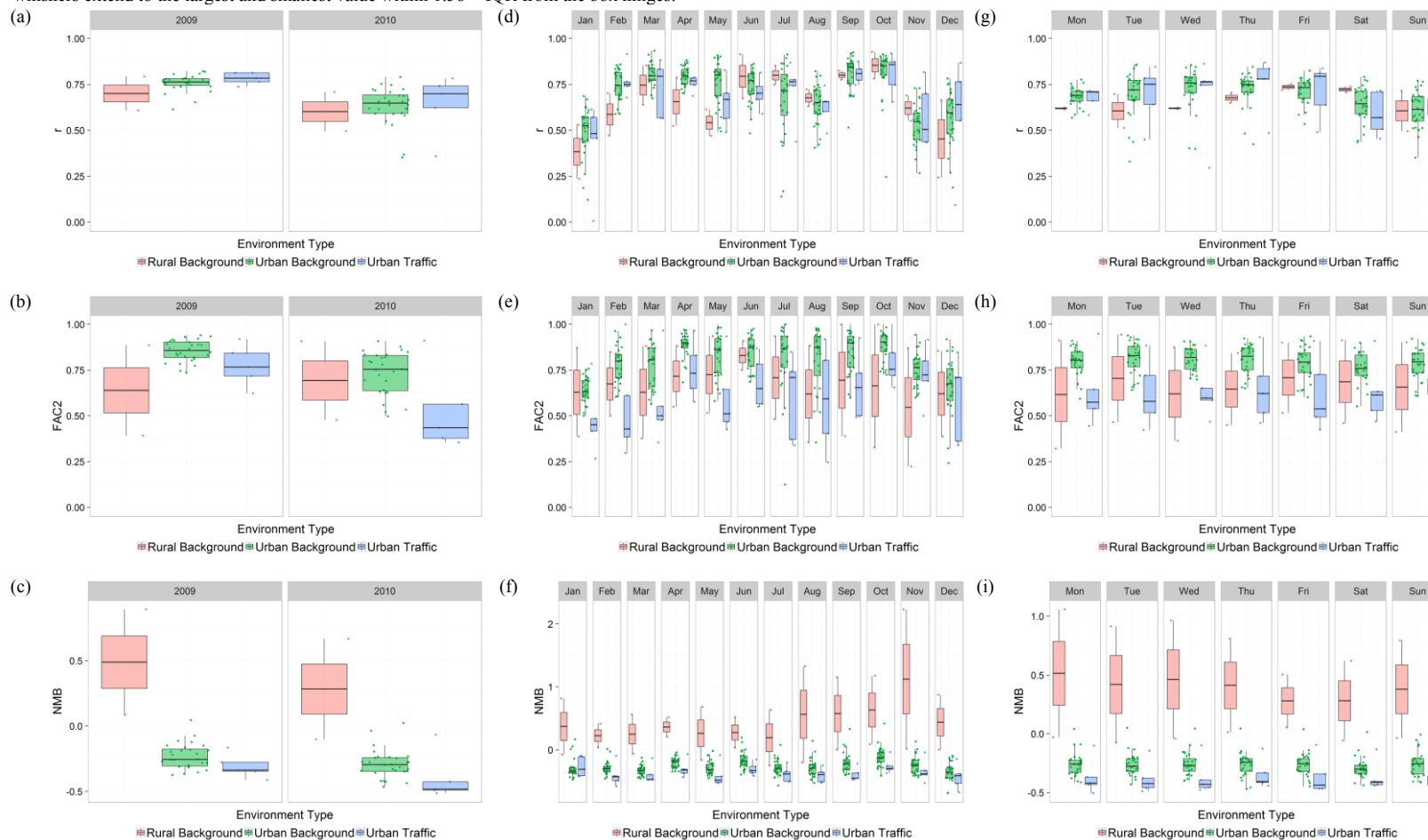
Figure 5: Model-measurement statistics per site for PM 2.5 daily mean concentrations during 2009-2010, by site type, and by (a-c) year, (d-f) month of year, and (g-i) day of week. (a), (d) and (g) are Pearson's correlation coefficient ( r ); (b), (e) and (h) are fraction of data pairs within a factor of two (FAC2); and (c), (f) and (i) are normalised mean bias (NMB). Dots show individual site statistics ( n = 2, 28 and 5 for RB, UB and UT sites respectively), which are summarised in the superimposed box-plot whose shading demarcates the interquartile range (IQR) and whose whiskers extend to the largest and smallest value within 1.58 \times IQR from the box hinges.
