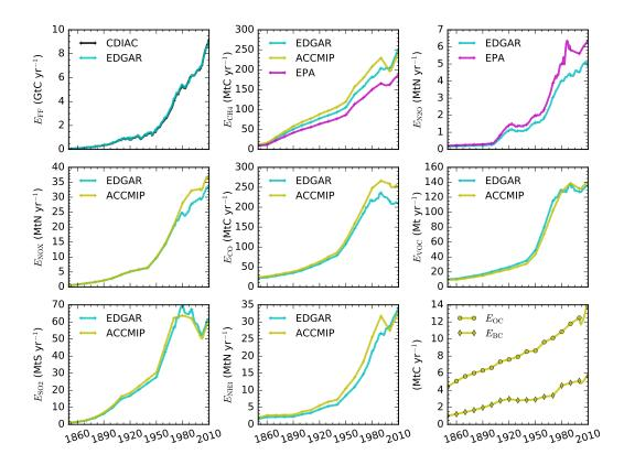
**Figure 2.** Time-series of the main anthropogenic emissions used as potential inputs of OSCAR (section 2.2.1). Other drivers of the model, i.e. emissions of halogenated compounds and LULCC, are shown in figure S1 and S2, respectively.
