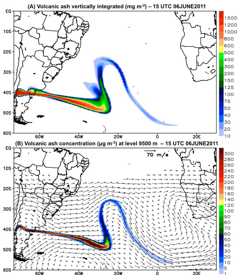
Figure 17. (A) Vertically integrated total mass of ash ( $\text{mg m}^{-2}$ ). (B) Total ash mass concentration ( $\mu\text{g m}^{-3}$ ) at level of approximately 9500 m above surface and the associated horizontal wind. Both panels show results for 15UTC 06 June 2011 as simulated by BRAMS model.
