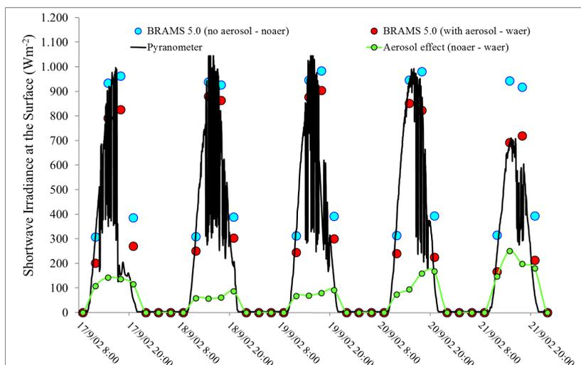
**Figure 2.** Time series of downwelling short-wave irradiance ( $\text{Wm}^{-2}$ ) at Abracos Hill AERONET site during a cloudy period from 17 to 21 September 2002 from BRAMS 5.2 results with (in red) and without (in blue) aerosol effects. The black line refers to measurement data in the same periods and the green (line and marks) is the attenuation due to aerosol effect.
