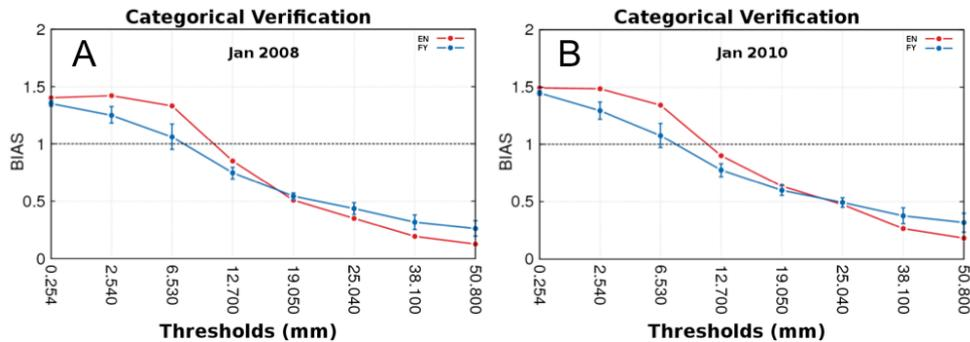
**Figure 5.** Mean bias score versus precipitation thresholds for South America for a set of 30 forecasts of 24-h accumulated precipitation for 120h in advance for (A) January 2008 and (B) January 2010.
