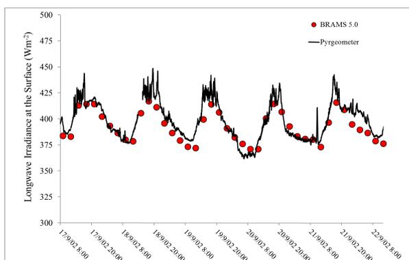
**Figure 3.** Time series of downwelling long-wave irradiance ( $\text{Wm}^{-2}$ ) at Abracos Hill AERONET site during a cloudy period from 17 to 21 September 2002 from BRAMS 5.2 results. The black line refers to measurement data in the same period.
