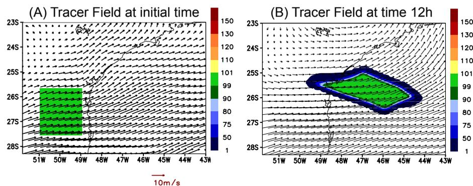
**Figure 1.** A 3-D hypothetical case study: transport of a rectangular parallelepiped by a realistic divergent flow over the Southeast part of Brazil. (A) The tracer concentration field expressed in terms of mass mixing ratio at initial time and 1900 m height; the horizontal wind flow is also depicted. (B) The correspondent mass mixing ratio after 12 hours as simulated by the monotonic advection scheme.
