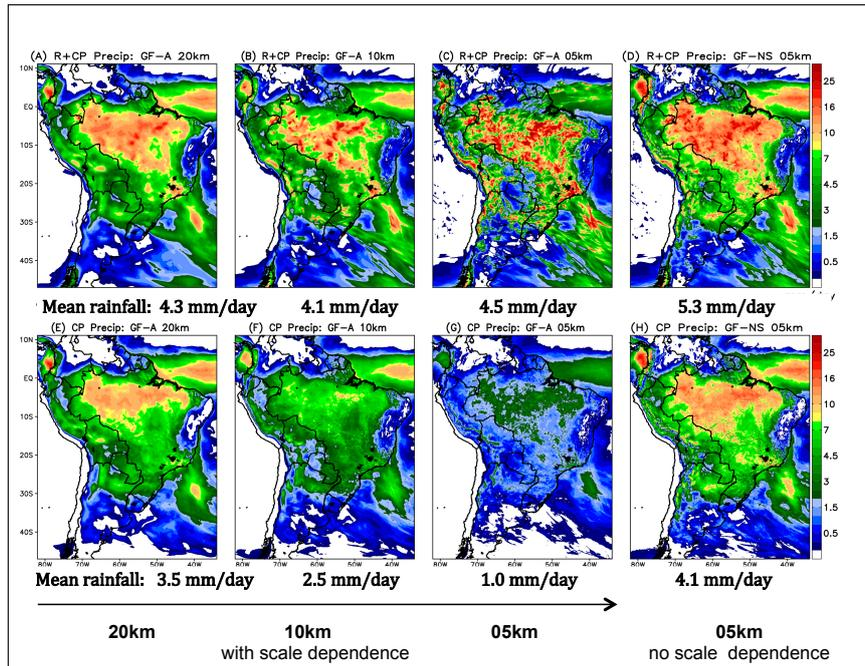
**Figure 6.** Averaged precipitation rates over 15 runs for total precipitation (A, B, and C) and convective (non-resolved) precipitation (E, F and G), using the scale dependence formulation (GF-A) and horizontal resolutions of 20km (A, E), 10km (B, F) and 5km (C, G). The column on the right (panels D and H) depicts results on 5 km without the scale dependence formulation (GF-NS). Units are mm/day.
