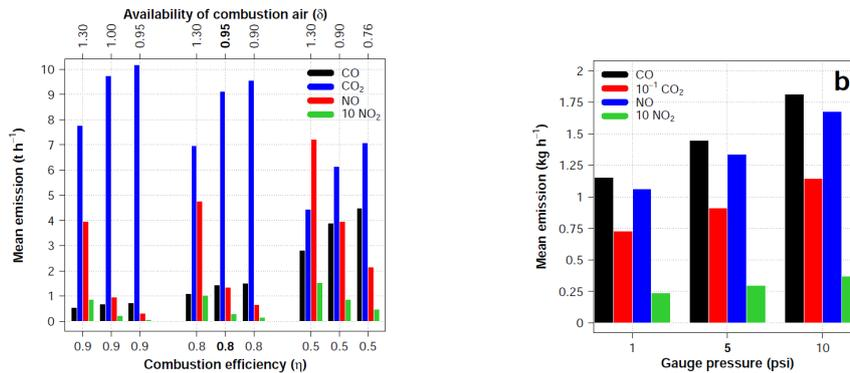
458 **Fig.8.** Flaring emissions ( $\text{kg h}^{-1}$ ) spatiotemporally averaged over SWA and TP15 depending on (a) combustion efficiency  $\eta$
