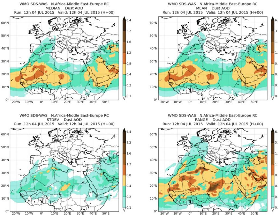
**Figure 8.** Dust AOD regional ensemble products valid at 12:00 UTC 4 July 2015. The multi-model products describing centrality (multi-model median and mean) and spread (standard deviation and range of variation) are generated from multiple global and regional forecast models, including NGAC V1.0. This figure is produced by the Regional Center for Northern Africa, Middle East and Europe of the WMO SDS-WAS program.
