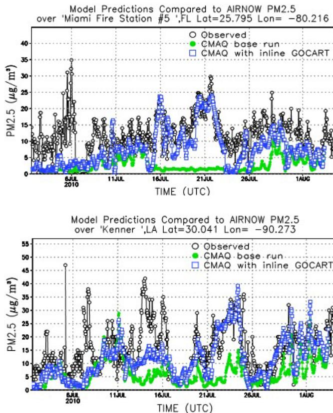
**Figure 9.** Time series of PM<sub>2.5</sub> from EPA AIRNOW observations (black dot), CMAQ baseline run using static LBCs (green dot) and CMAQ experimental run using NGAC LBCs (blue square) at Miami, FL (top panel) and Kenner, LA (bottom panel).
