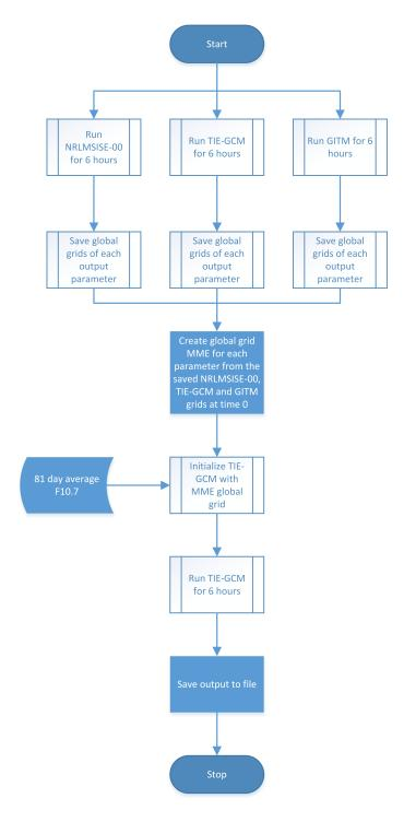
**Figure 12.** Flow chart of the procedure for running TIE-GCM using the MME as its initial conditions for a six hour forecast.
