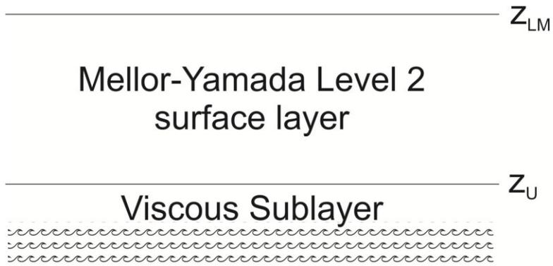
Figure 2. The Mellor-Yamada surface layer with the viscous sublayer over the ocean. The symbol  $Z_{LM}$  is the height of the lowest model layer and  $Z_U$  is the depth of the viscous sublayer for momentum. (Reproduced from Janjic, 1994).
