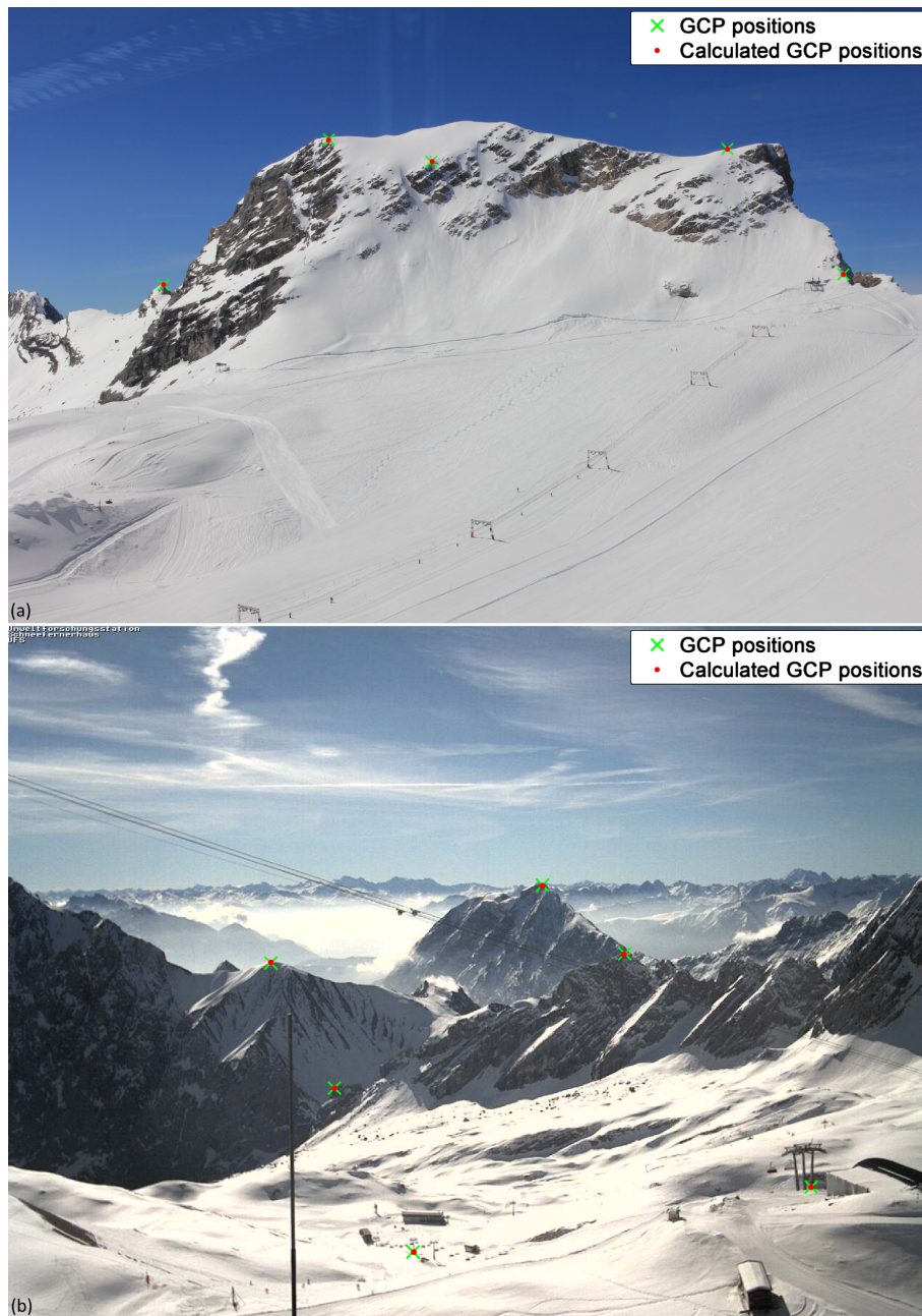
Figure 9. Real and calculated GCP positions for the investigated photographs on 7 April 2014: the root mean square error (RMSE) between real (green crosses) and calculated (red dots) GCP positions are 0.5 m for the SLR photograph (a) and 2.2 m for the webcam photograph (b) after the optimisation of the camera parameters.
