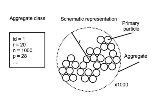
**Figure 1.** A schematic of an AC. The complete list of attributes is in Table 1. The AC in this example represents 1000 aggregates each composed of 28 primary particles.
