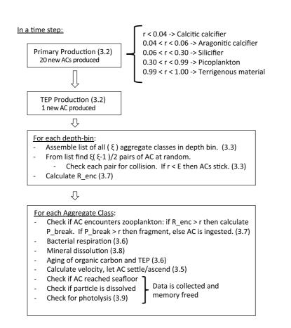
Figure 4. An outline of what the model does in a timestep. In parenthesis are the sections where each task is explained.
