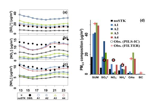
**Figure 9.** Time-series comparison of 1 h averaged **(a)**  $SO_4^{2-}$ , **(b)**  $NO_3^-$ , and **(c)**  $NH_4^+$  concentrations measured from PILS-IC instrument and model-predicted concentrations. In panel **(d)**, 24 h averaged aerosol concentration in  $PM_{2.5}$  from observations (PILS-IC instrument and low air volume sampler with Teflon filter) are compared with hindcast concentrations at the Yongin City site for ten selected episodes.
