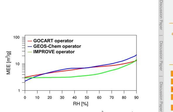
**Figure 4.** Mass extinction efficiencies (MEEs) calculated for  $SO_4^{2-}$ ,  $NO_3^{-}$ , and  $NH_4^+$  at a wavelength of 550 nm as a function of relative humidity (%) from three observation operators.
