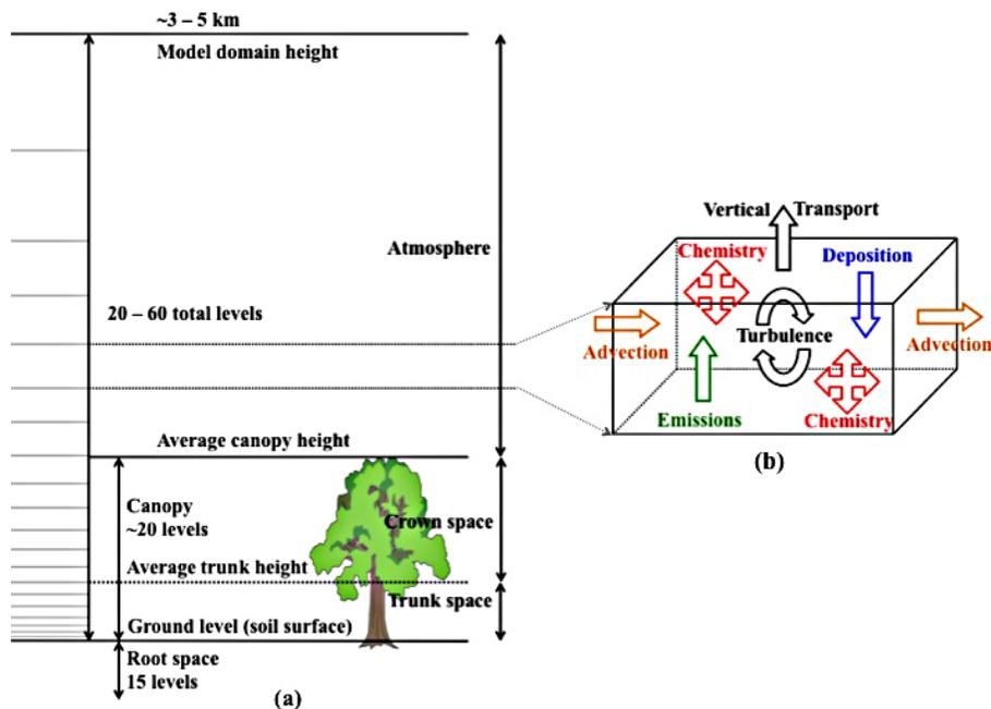
**Figure 1.** (a) A schematic of the FORCAst column model. Each level within the column is a box model (b) incorporating the processes involved in canopy-atmosphere exchange of energy and mass appropriate for that level.
