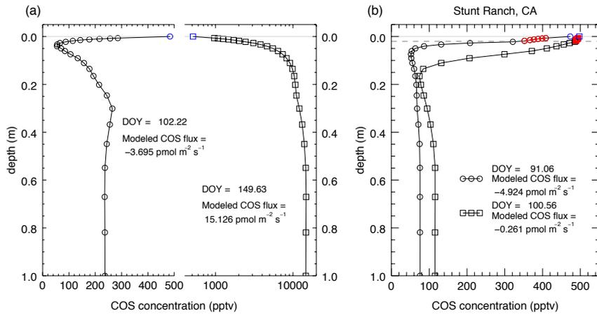
**Figure 7.** Typical simulated profiles of COS concentration. (a) COS profiles of a strong uptake case (circles) and a strong emission case (squares) at SGP. The right side of the  $x$ -axis is on logarithmic scale. (b) COS profiles during the wet period (circles) and the dry period (squares). Blue color is used for the atmospheric concentrations, and red for the concentrations in the litter layers in (b).
