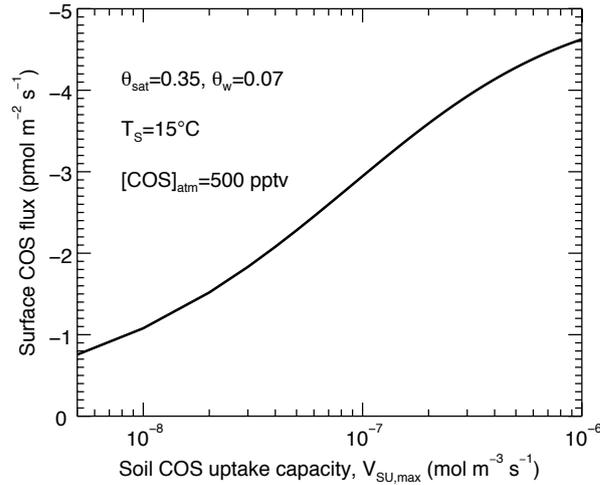
**Figure 10.** An idealized numerical experiment to test the sensitivity of COS flux to soil COS uptake capacity, with  $\theta_{sat} = 0.35$  m<sup>3</sup> m<sup>-3</sup>,  $\theta_w = 0.07$  m<sup>3</sup> m<sup>-3</sup>, soil temperature at 15°C, and ambient COS concentration at 500 pmol mol<sup>-1</sup>. Note that the  $x$ -axis is in logarithmic scale and the  $y$ -axis is reversed for showing COS uptake.
