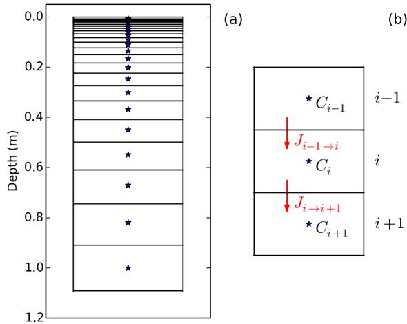
**Figure 1.** (a) The vertical finite-volume boxes and computational nodes (asterisk). (b) A schematic figure showing the diffusive fluxes ( $J$ ) across boxes, which relate to concentration changes through mass balance.
