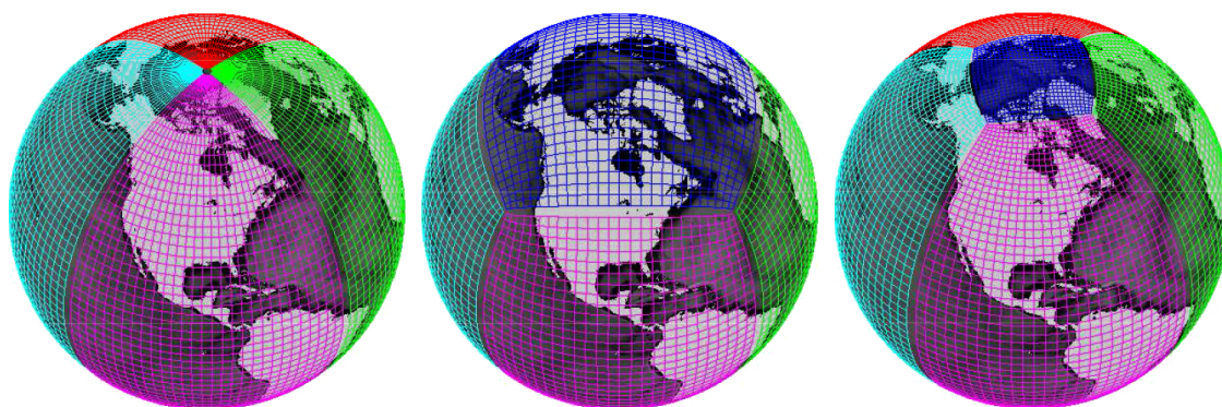
Figure 1. Three possible approaches to gridding the Globe. Left: LL maps the earth to a single rectangular array (one face ). Center: CS (six faces). Right: LLC (five faces). The faces of CS and LLC are color-coded; LL is only split four ways for rendering. Acronyms are defined in Sect. 2.
