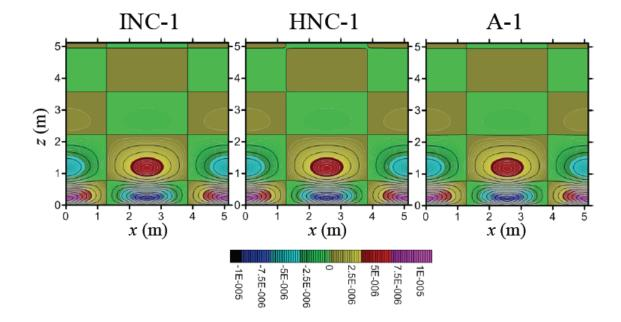
Figure 3. Vertical cross section of u from the first test case. A-1 is the analytical solution. INC-1 is the numerical simulation with inhomogeneous Neumann condition pressure. HNC-1 is the numerical simulation with the homogeneous Neumann condition for pressure. Color bar units are m s<sup>-1</sup>.
