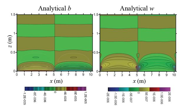
**Figure 4.** Vertical cross section of the analytical (A-2) buoyancy b and vertical velocity w fields from the second test case. Color bar units are m s<sup>-2</sup> for b, and m s<sup>-1</sup> for w.
