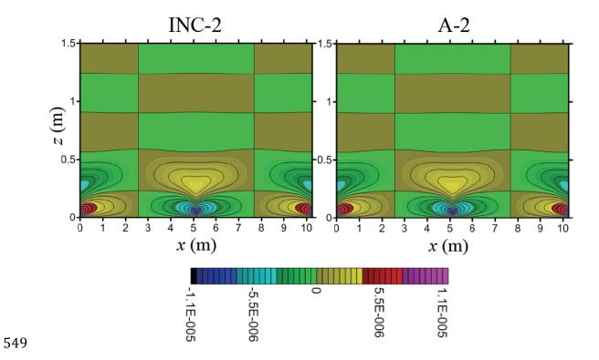
**Figure 5.** Vertical cross section of u from the second test case. A-2 is the analytical solution. INC-2 is the numerical simulation with inhomogeneous Neumann condition for pressure. Color bar units are m s<sup>-1</sup>.
