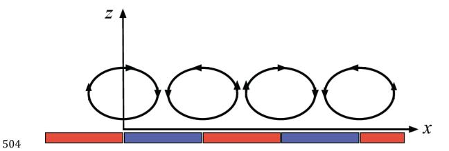
**Figure 1.** Schematic of two-dimensional (x, z) thermal convection induced by a surface buoyancy that varies horizontally (x) as a square wave. Red denotes positive surface buoyancy, blue denotes negative surface buoyancy.
