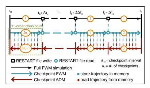
Figure 4. Second order checkpointing scheme implemented in WRFPLUS-Chem.
