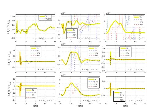
**Figure 5.** Time variant sensitivities of cost function J with respect to control variable x for multiple perturbations and the TLM with second order checkpointing.
