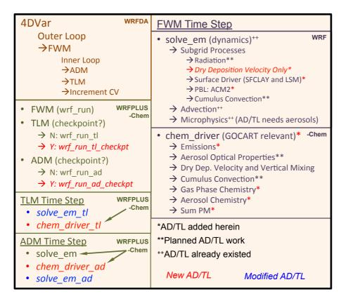
**Figure 1.** Dependencies between WRF, WRF-Chem, WRFPLUS AD/TL, and WRFDA. AD/TL development status is also noted.
