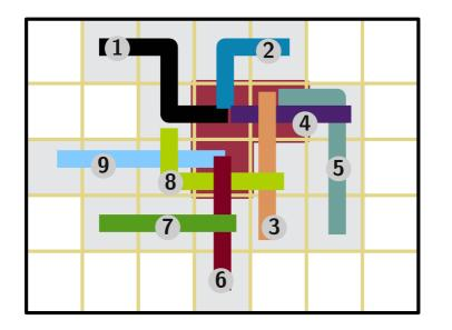
**Figure 8.** Schematic example of a region of low probability values caused by many members. Of nine members that predict the WCB feature, only a maximum of three overlap in any grid cell. By storing the indices of all members that contribute to a given grid cell, our method is able to determine the members that contribute to a probability region.
