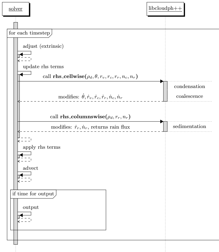
Figure 5. Sequence diagram of libcloudph++ API calls for the double-moment bulk scheme and a prototype transport equation solver. Diagram discussed in Sect. 4.2.2. See also caption of Fig. 2 for description or diagram elements.
