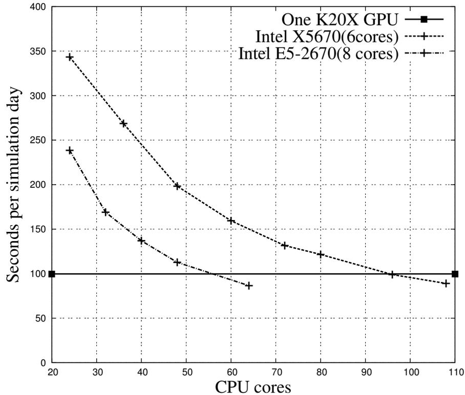
Figure 8. Performance comparison with different hardware platform.
