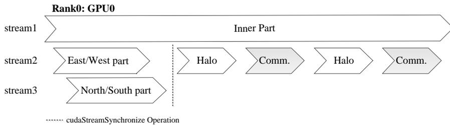
**Figure 4.** The workflow of multiple streams on the GPU. The “inner/east/west/north/south part” and “Halo” refer to computation and update of corresponding part. “Comm.” refers to communication between processes, which implies synchronization.
