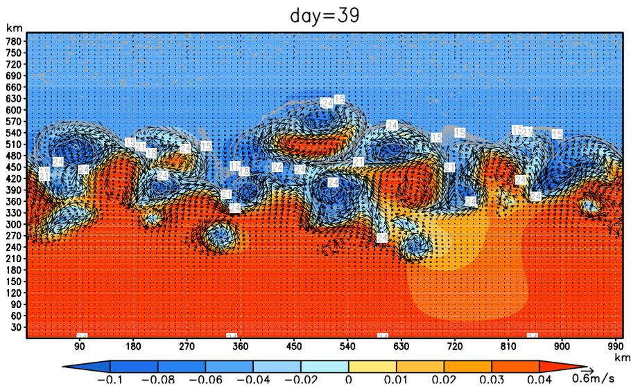
**Figure 7.** The sea-surface height (SSH), sea-surface temperature (SST), and currents after 39 days simulation.
