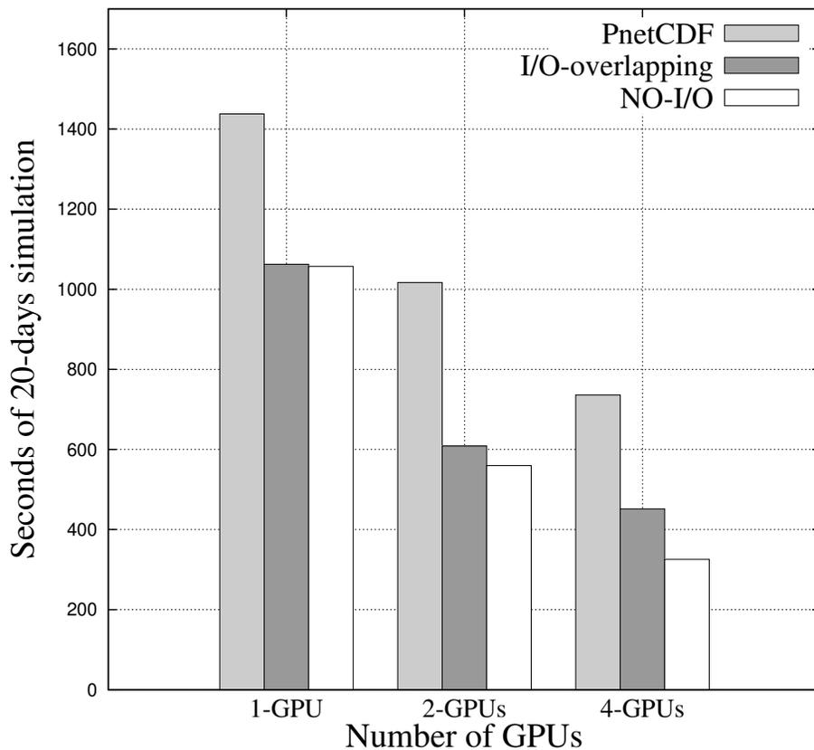
Figure 10. I/O Test for gpuPOM.
