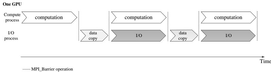
**Figure 6.** One computing process and one I/O process both set their contexts on the same GPU. During the data copy phase, the computing process remains idle and the I/O process will copy data from the GPU to the CPU host through the cudaMemcpy function.
