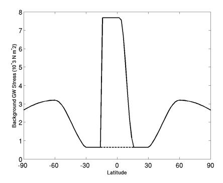
**Fig. 3.** Background nonorographic drag from the MERRA (dashed line) and MERRA2 AGCM (solid line) simulations. The dashed line underlies the solid line outside of the tropics.
