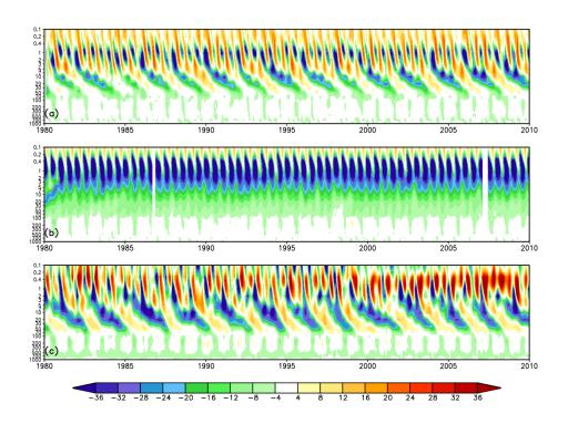
Fig. 4. Spatial average of zonal wind in  $m s^{-1}$  from 10S to 10N latitude as a function of pressure level in mb and time from a) MERRA2 AGCM control, b) Experiment 2 and c) MERRA reanalysis.
