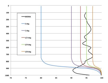
**Fig. 7.** Critical relative humidity. Black from MERRA AGCM formulation, blue from MERRA2 AGCM formulation for  $2^{\circ}$  resolution, purple from MERRA2 AGCM formulation for  $1^{\circ}$  resolution, brown from MERRA2 AGCM formulation for  $1/2^{\circ}$  resolution, green from MERRA2 AGCM formulation for  $1/4^{\circ}$  resolution, orange from MERRA2 AGCM formulation for  $1/8^{\circ}$  resolution.
