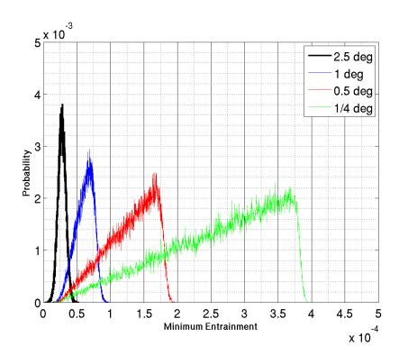
Fig. 17. The probability distribution function for the minimum entrainment allowed by the cumulus parameterization for different AGCM horizontal resolutions. Black line is for 2x2.5 degree, blue for 1 degree, red for 1/2 degree and green for 1/4 degree.
