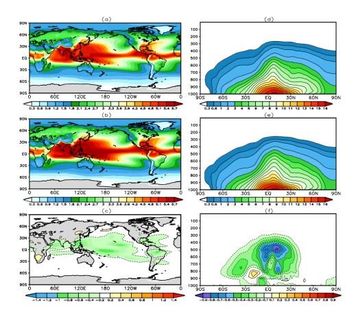
**Fig. 14.** a) June-July-August total precipitable water in mm from experiment 6 (MERRA AGCM-like), b) same as a) but from experiment 5, c) same as a) but the difference, experiment 6 minus experiment 5, d) June-July-August specific humidity in  $g kg^{-1}$  from experiment 6 (MERRA AGCM-like), e) same as d) but from experiment 5, f) same as d) but the difference, experiment 6 minus experiment 5.
